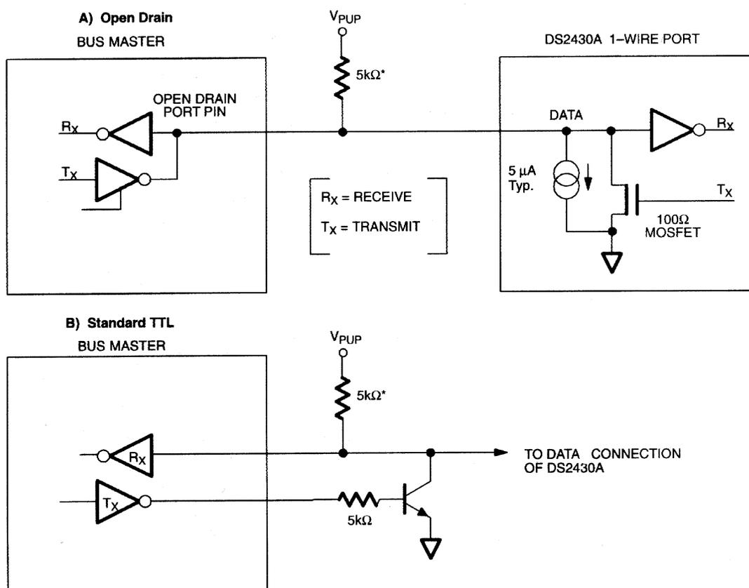
\*5 k $\Omega$  is adequate for reading the DS2430A. To write to a single device, a 2.2 k $\Omega$  resistor and  $V_{PUP}$  of at least 4.0V is sufficient. For writing multiple DS2430As simultaneously or operation at low  $V_{PUP}$ , the resistor should be bypassed by a low-impedance pullup to  $V_{PUP}$  while the device copies the scratchpad to EEPROM.
