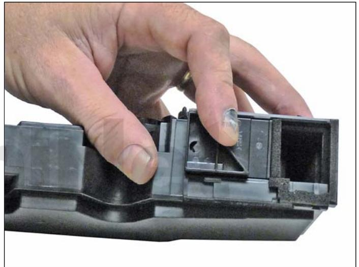
3. Remove the waste chamber. Slide the cover open and vacuum/blow the waste chamber clean.
