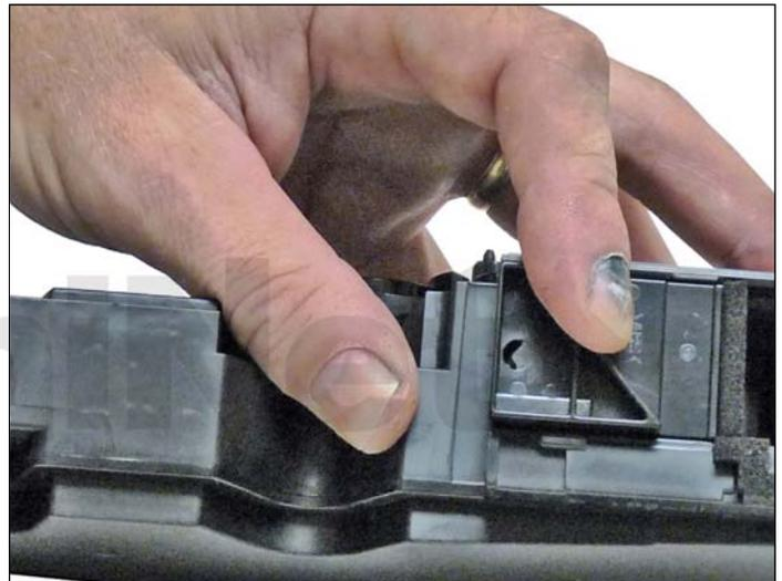
11. Remove the waste chamber. There are two small gears that will come loose.
