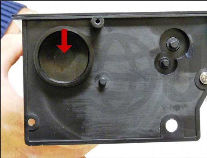
12. Remove the toner fill plug. Dump the bulk of the remaining toner out of the cartridge. Vacuum/blow out the toner supply chamber clean.
