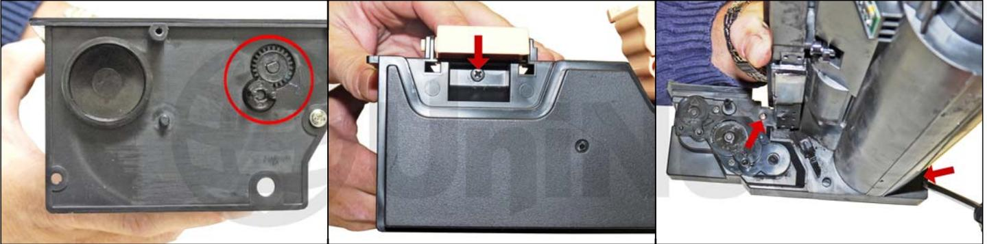
14. Install the two gears on the hopper. Install the waste chamber and three screws.
