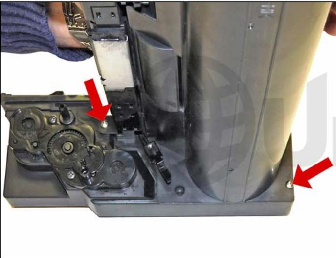
1. Remove the two screws located on the waste chamber.
