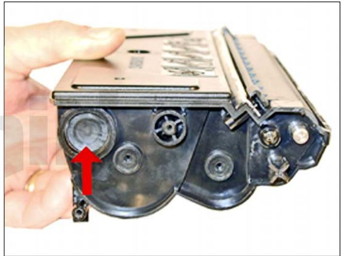
19. Install the fill plug. Check for leaks.
