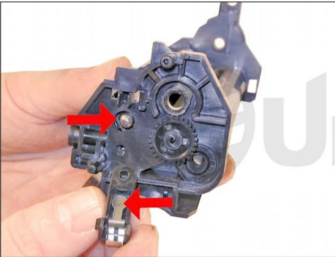
14. Place a small amount of conductive grease on the tip of the PCR shaft. Clean all the old conductive grease from the contact plate, and replace it with new grease. Install it on the cartridge and install the screw.
