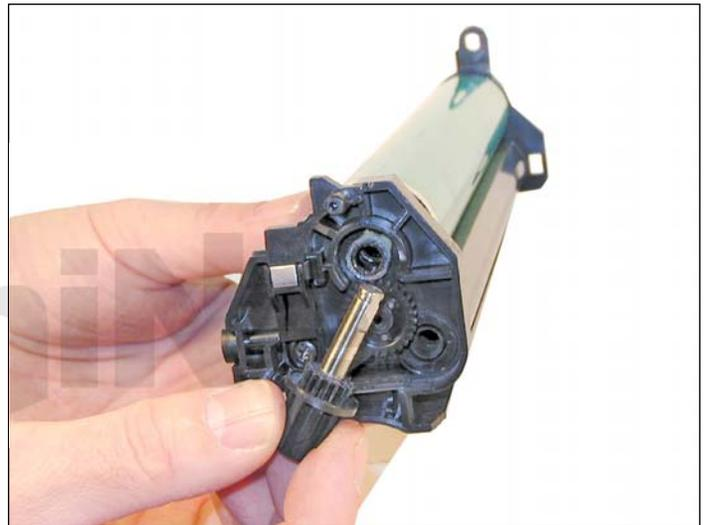
17. On the left side of the cartridge, install the drum drive gear and axle. Make sure the teeth of the gear mesh properly.
