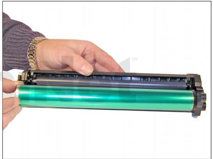
15. Install the drum gear side to the right. As with the wiper blade, the OEM drum if in good shape should run another cycle. Further than that is not a good idea.
