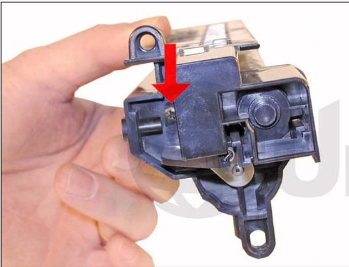
19. Install the waste chamber, and screw.
