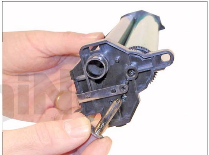
4. Remove the screw on the drum axle and the drum axle pin.
