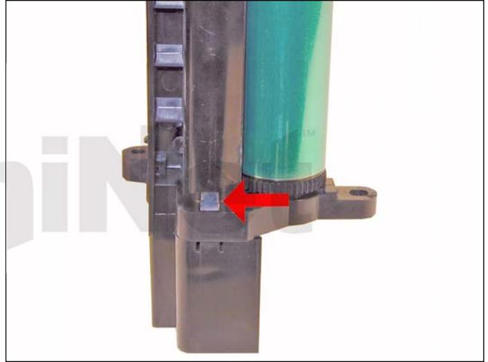
1. Remove the screw located on the waste chamber.
