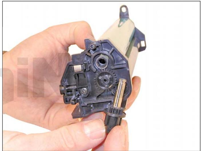
5. On the opposite side of the cartridge pry out the drum drive gear and axle pin from the drum.
