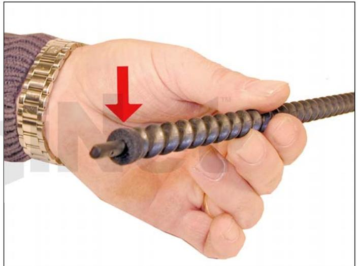
3. Vacuum the auger and foam seal clean.
