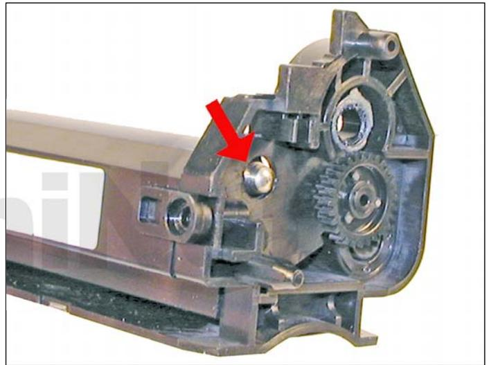
13. Install the PCR assembly right side first.
