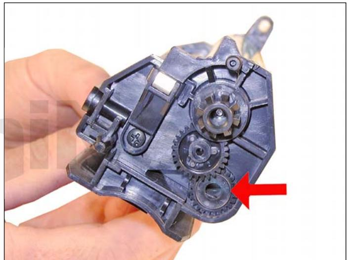
2. Remove the waste auger from the cartridge. The augers drive gear will come loose at this point.
