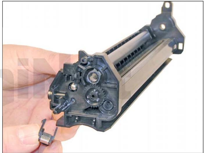
7. On the right side of the cartridge, remove the screw and contact insert.
