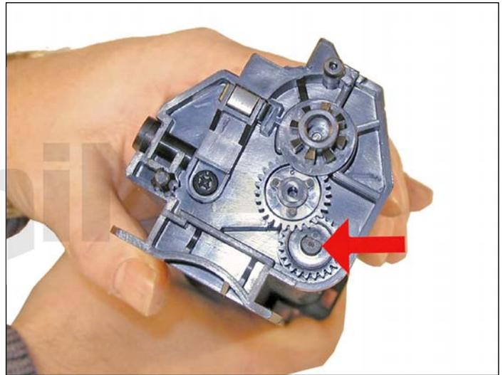
18. On the gear side, install the auger drive gear under the middle gear.
