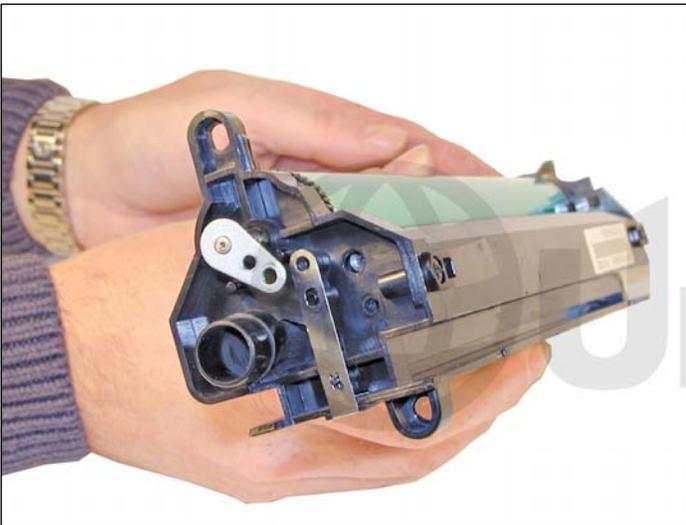
16. Clean the old conductive grease off the drum axle pin. Place new grease on the shaft, and install into the cartridge. Install the axle screw.
