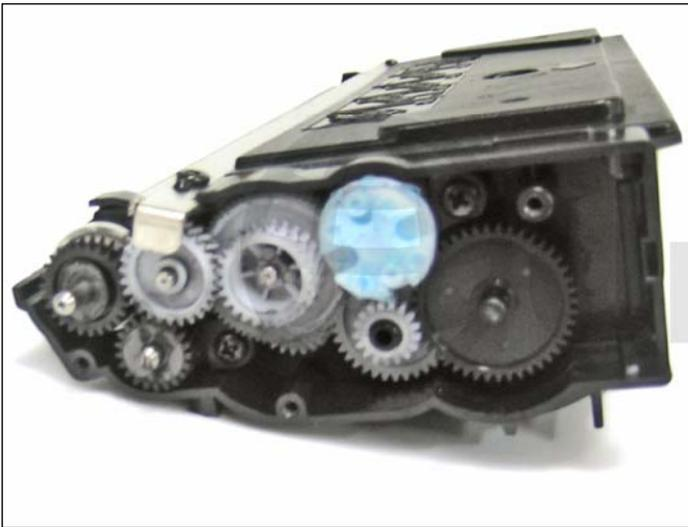
13. Remove the rest of the gears shown.
