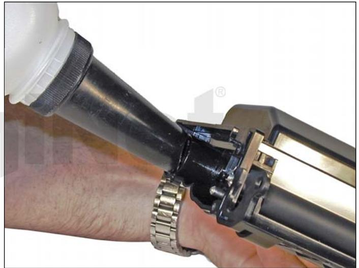
21. Fill the hopper with 135g or 290g of toner for use in Xerox WorkCentre 3550. Check for leaks.
