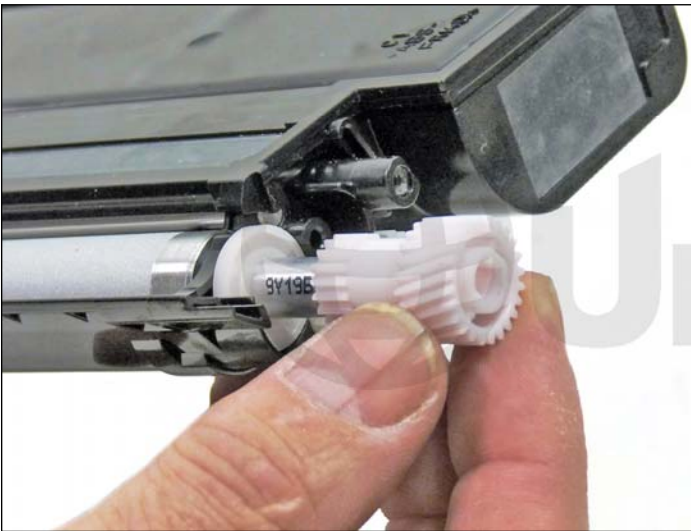
9. Remove the large mag roller drive gear.
