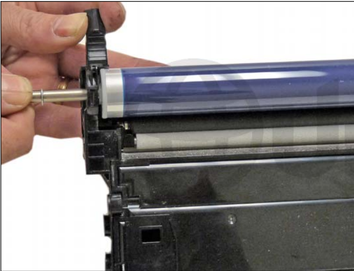
37. Install the drum axle from the hub side.
