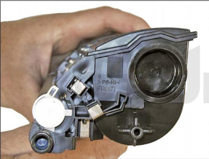
1. Remove the fill plug, and dump out any remaining toner.
