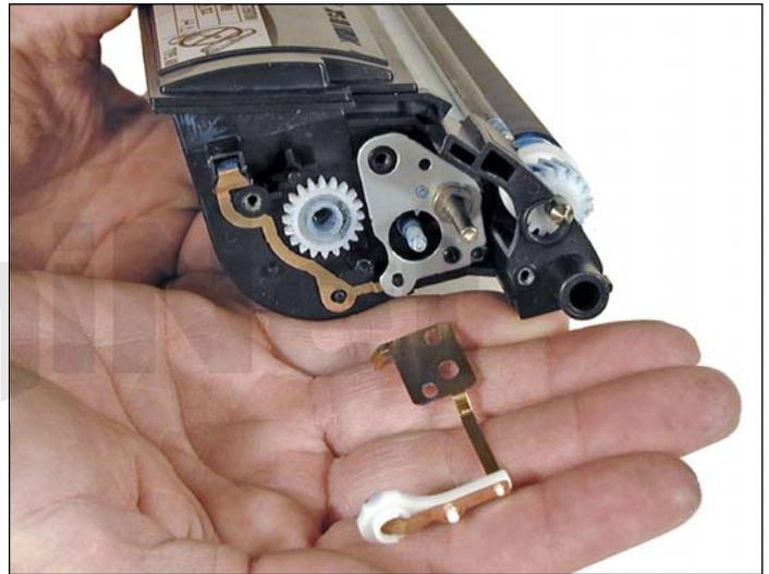
6. Remove the contact/bushing assembly.
