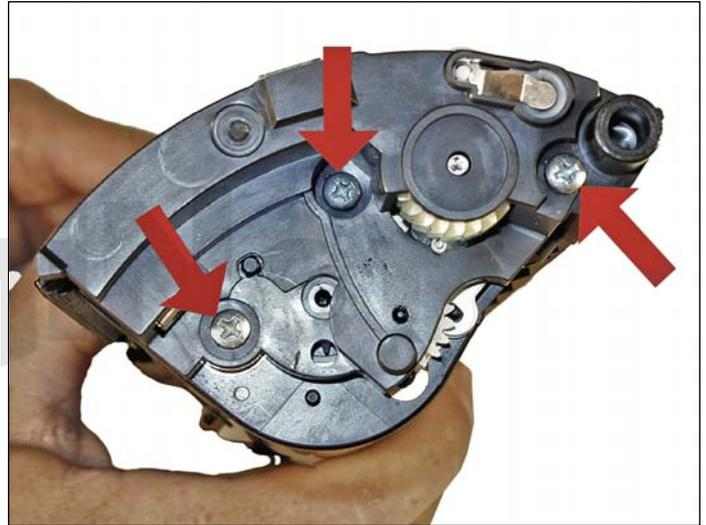
2. On the gear side of the cartridge, remove the three silver screws from the end cap.
