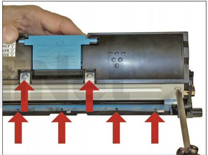
17. Install the cleaned sealing blade assembly, seals, contact, and three screws. Make sure the foam aligns with the plastic pins.
