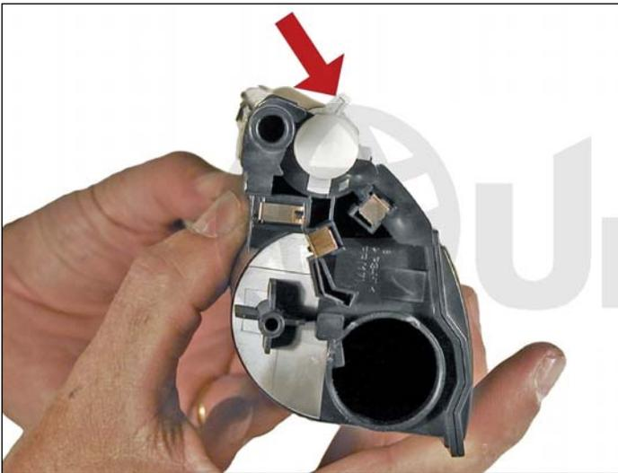
7. Remove the white bushing from the non-gear side by prying up the center tab and rotating the bushing counter-clockwise until it stops. Pry the bushing off the developer roller shaft.
