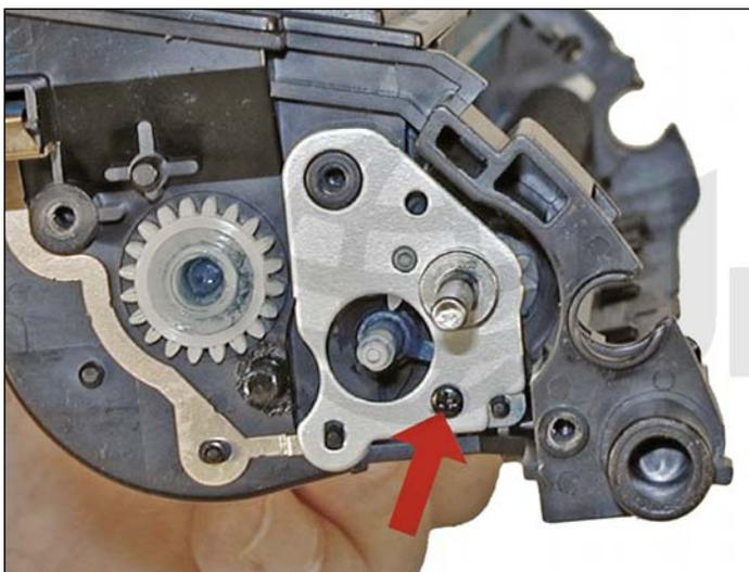
14. Remove the small screw from the feed roller contact plate, and remove the plate.
