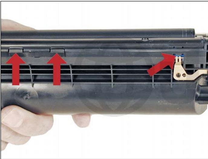
8. Remove the doctor blade cover by prying up the three tabs as indicated. Remove the cover.
