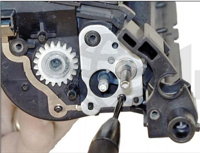
16. Re-install the feed roller contact plate and screw.
