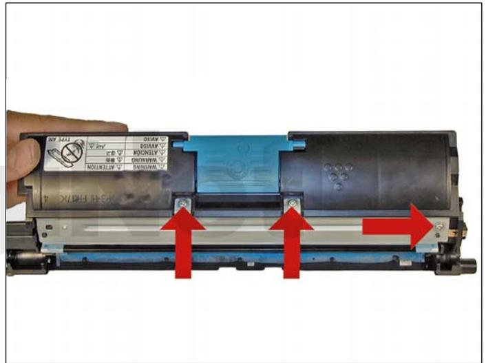
11. Remove the three screws on the sealing blade assembly.
