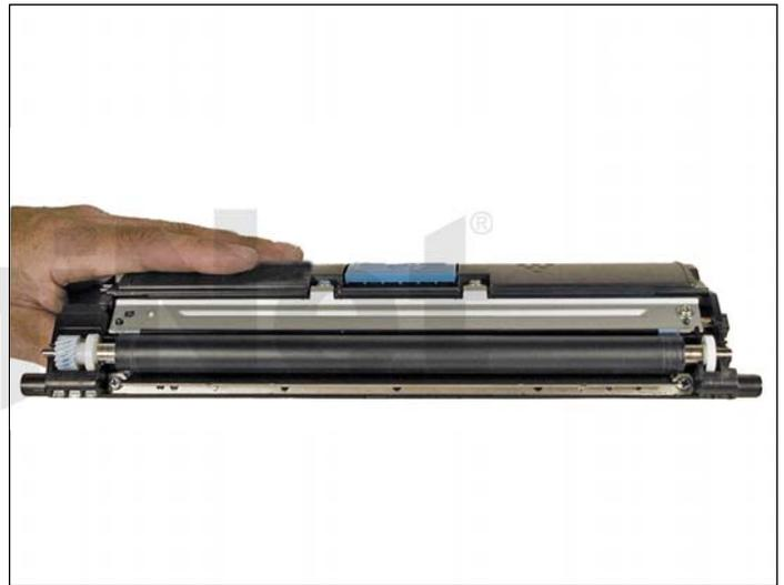
19. Install the developer roller assembly.
