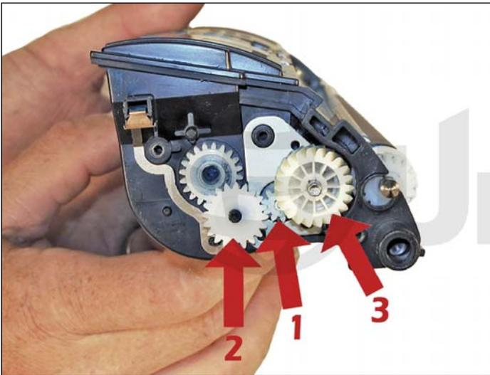
21. Install the three gears smallest to largest in that order.
