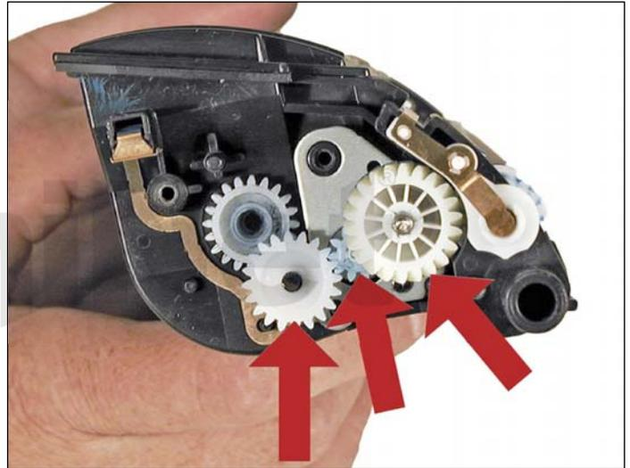
4. Remove the larger drive gear and the two smaller gears next to it. Leave the mixing blade gear in place.
