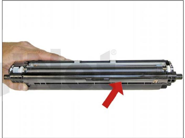
24. Install the doctor blade cover. Rotate so that the tabs are aligned and snap in place. This may take a bit of force to fit properly.
