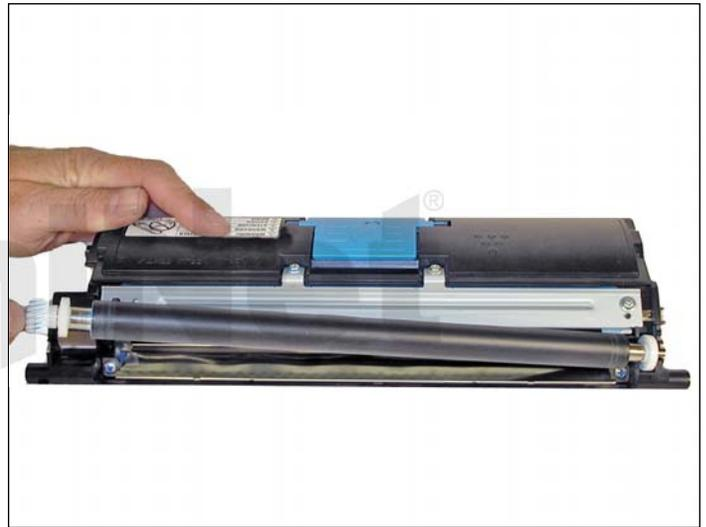
9. Remove the developer roller and gears.
