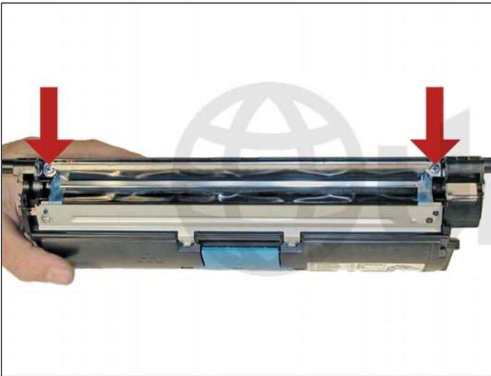
18. Install the doctor blade and two screws.
