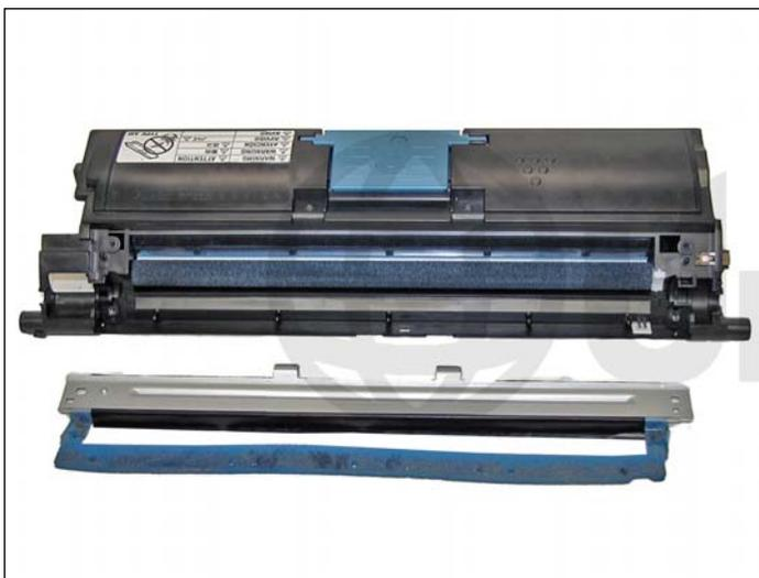
12. Pry up the sealing blade assembly and lift off.
