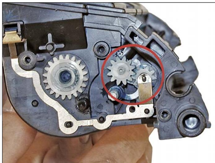
15. Check to ensure that the contact to the feed roller is clean, and that the two gears are clean and greased. If not, clean them and re-grease the gears with white lithium grease.
