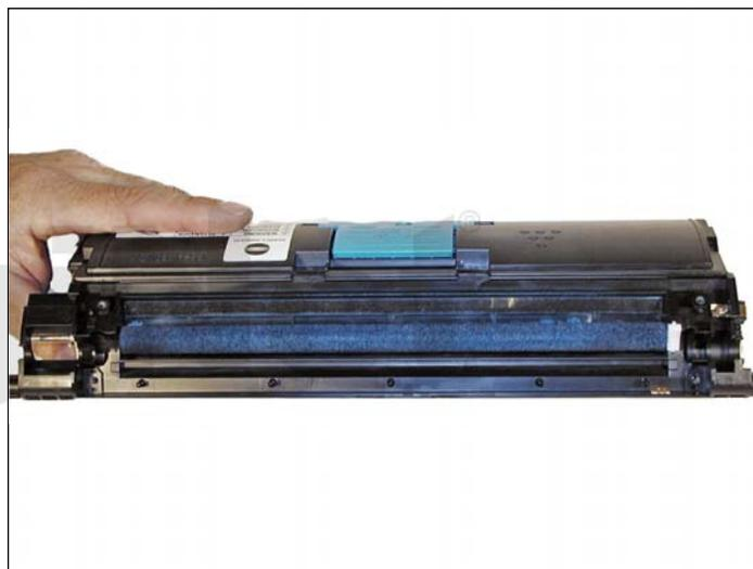
13. Clean out any remaining toner from the hopper and the feed roller.
