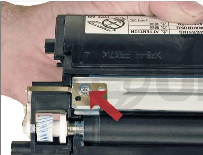
5. Remove the doctor blade contact screw.
