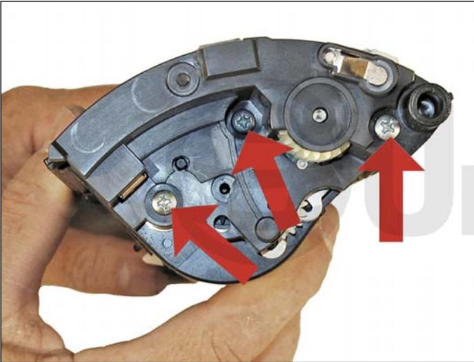
23. Install the black end cap on the gear side.
