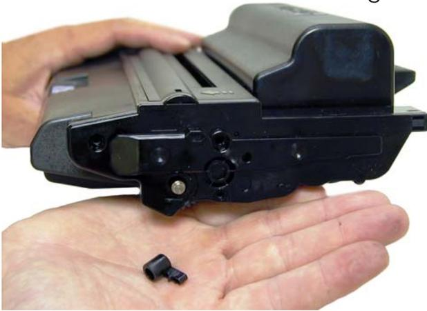
6) On the top edge of the end cap, there is a plastic tab. Press in on the tab and remove the left end cap. See **Figures 8 & 9.**
