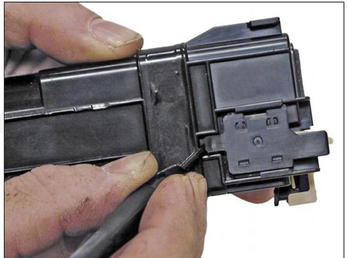
8. Carefully pry up the plastic chip holder tab.
