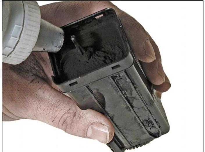
4. Fill the hopper with the appropriate replacement color toner. Remember, while the cartridges all look the same, they are not interchangeable. Each color has a different set of plastic tabs.
