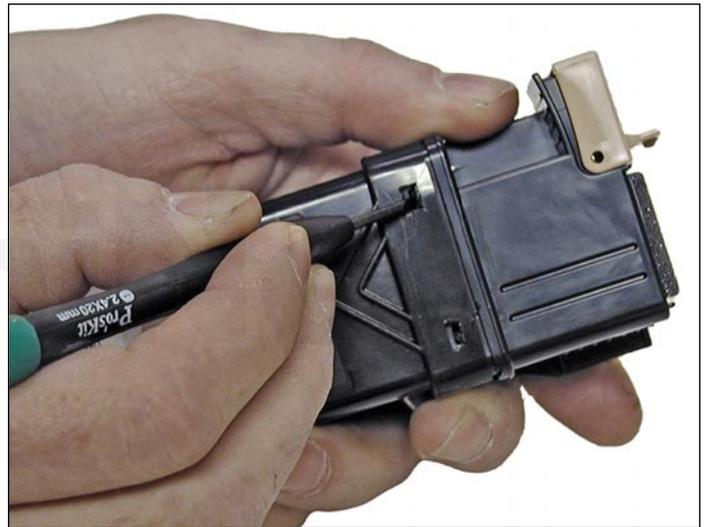
2. Press in on the two tabs of one side as shown to release the waste chamber. It is sometimes helpful to press back on the waste chamber as the tabs are pressed in.
