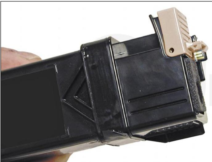
7. Re-install the black tape seal across the seam. If the OEM tape is not useable, good black rubber electrical tape (NOT the vinyl type) will work fine (toner will stick to anything made from vinyl).
