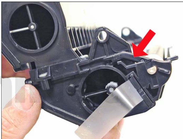
28. Clean the magnetic roller assembly with a dedicated magnetic roller cleaner.
