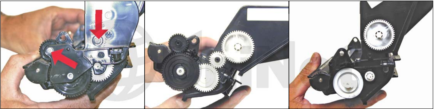
16. On the side opposite the fill plug, remove the two screws and end cap and gears as shown.
