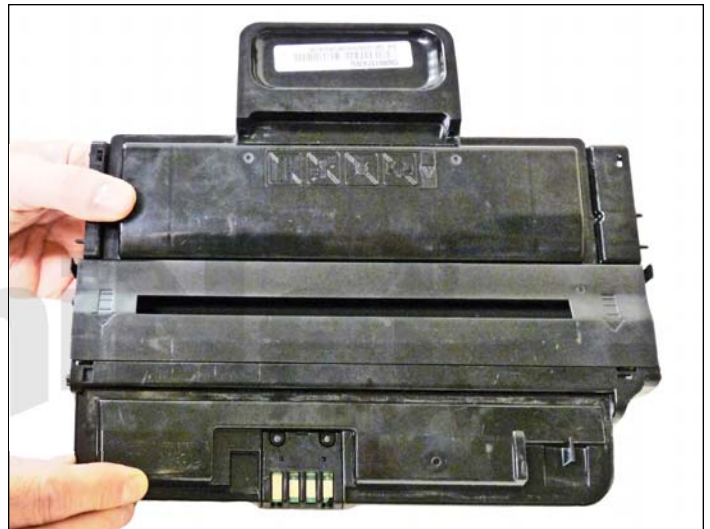
28. Slide the middle top cover/PCR assembly into place. Make sure all the middle tabs fit under the edge of the waste hopper.
