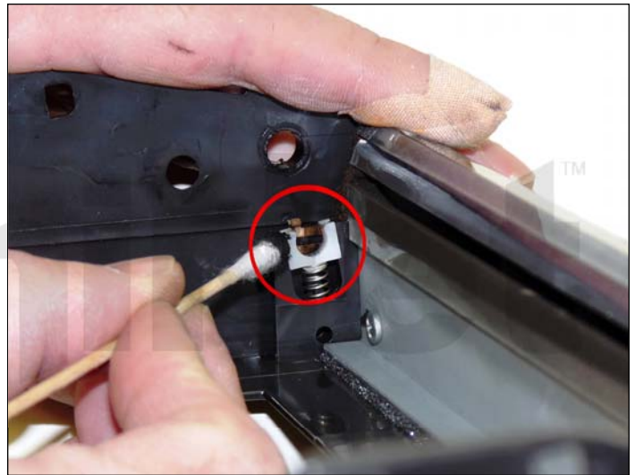
8. Clean off all the old conductive grease from the PCR contacts and replace with new. Remember: whenever using conductive grease more is never better. Only use a small amount (match what the OEM had there).
