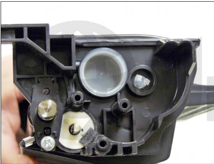
14. Remove the gear from the fill plug area by pressing in on the tab.
