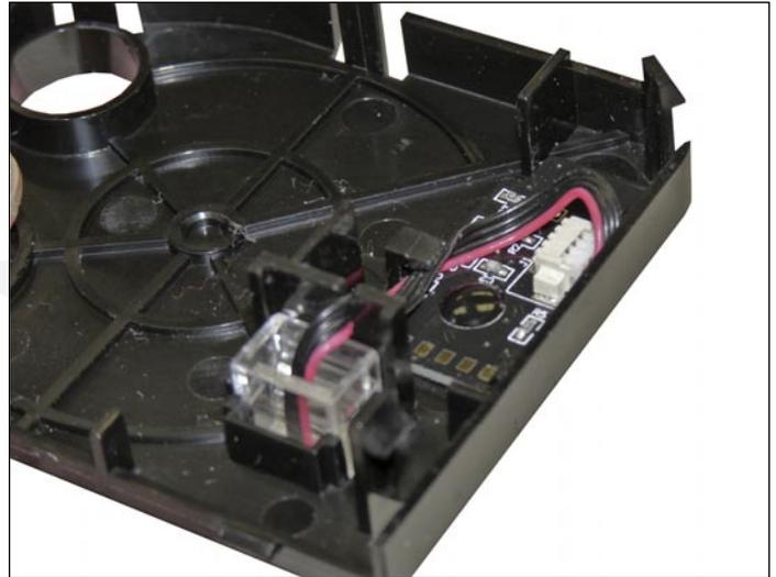
10. Replace the chip on the cartridge.
