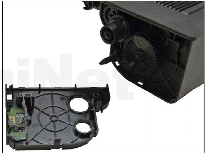
9. Press in on the four tabs on the opposite side of the cartridge.
