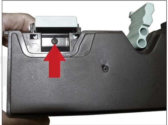
2. Remove the screw that is located under the colored plastic handle.
