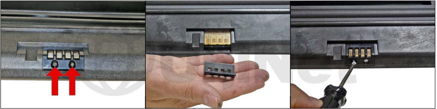
39. The chip is held in place by plastic rivets. It must be replaced for the cartridge to work.
