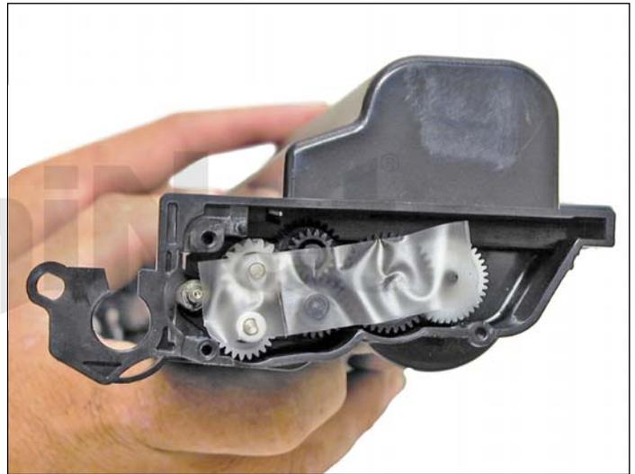
11. Remove the developer roller drive gear; place a strip of tape across the remaining gears as they do not need to be removed.
