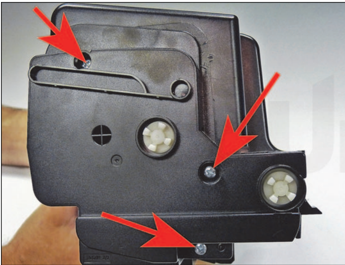
1. Remove the three screws from the drive gear (right) side end cap.
