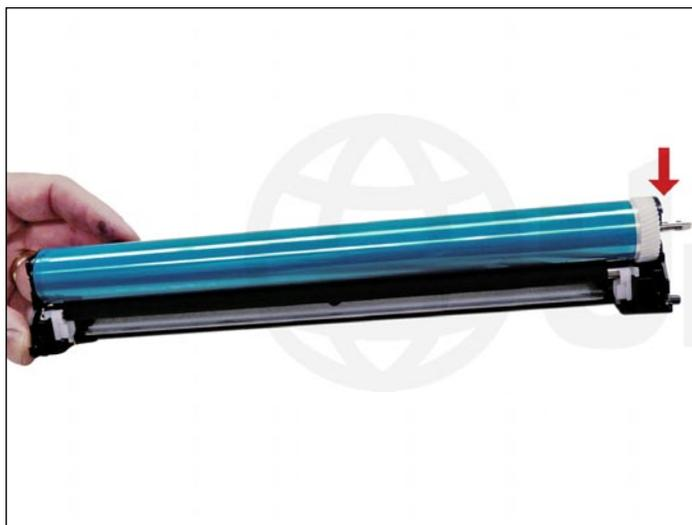
20. Install the drum into the waste hopper.
