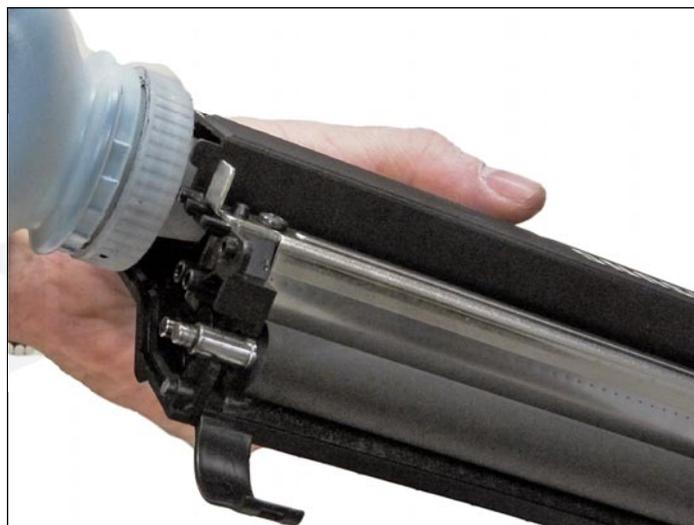
29. Fill the hopper with new replacement toner for use in the Samsung ML-2955. Replace the fill plug and check for leaks.
