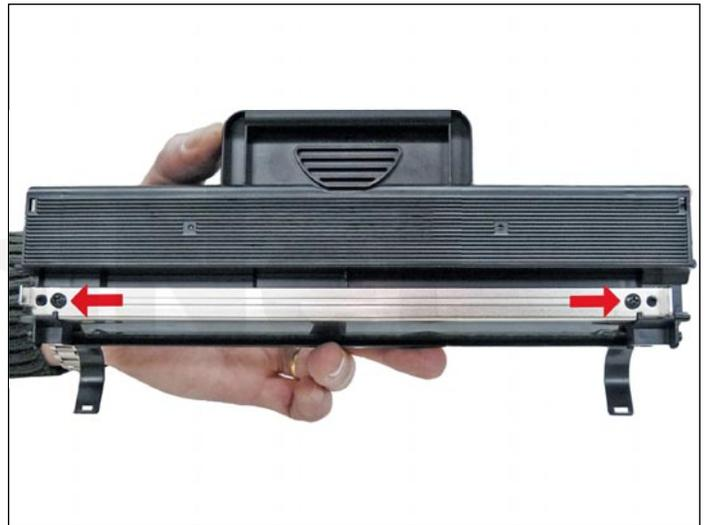
27. Install the doctor blade and two screws.
