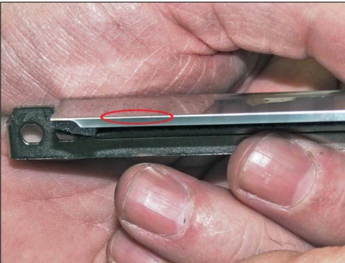
26. Clean the edge of the doctor blade, so there is no evidence of build up along the edge. If any build up exists, the cartridge will streak. No chemicals should be used. We have found that using a clean ice cream-type wooden stick works great for scraping the blade clean without damaging it.
