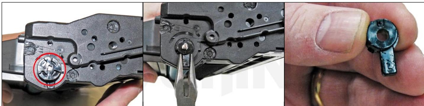
5. On the drum gear-side end cap, remove the drum drive-gear and the remaining arm the same way as the right side. Turn it to be straight down, and pull it straight out. Press in on the top tab and bottom tabs and remove the end cap. Note that the arm is stamped with the letter "L" to indicate the left side of the cartridge.
