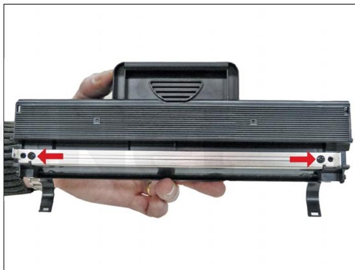
23. Remove the two screws from the doctor blade, and remove the blade.
