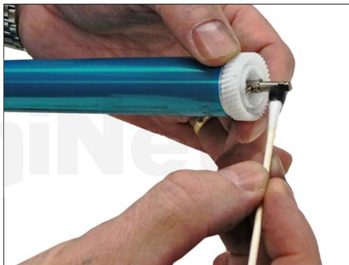
19. The drum axle shaft, on the large gear-side of the drum, has conductive grease on it. Regardless if you are replacing the drum or not, clean the old grease off, and replace with new.
