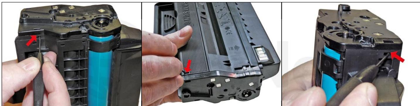
4. While still on the contact-side end cap, locate the top, bottom, and front tabs.
