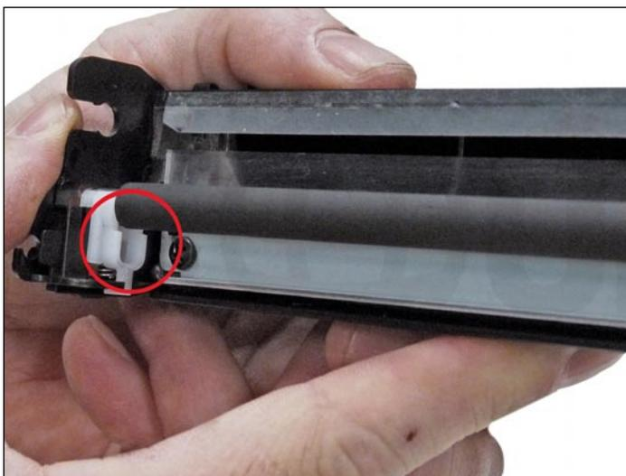
18. Place a small amount of conductive grease in the PCR holders, and install the PCR. Note that there is a place on the holders for a PCR-cleaning roller. It is not used in the cartridge. Samsung seems to be using parts from other cartridges for the D103.
