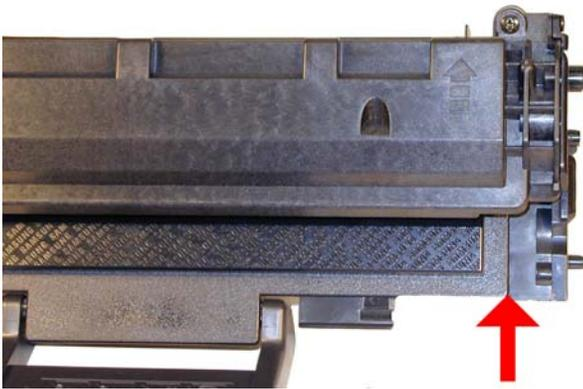
31) If your cartridge has a fuse, it needs to be replaced. Replace the fuse located on the right front of the cartridge (with the handle away from you). The ML-2010 does not use a fuse, and no other machines/cartridges are available yet (9/2005), but the slot for a fuse is there so it is possible that some of these cartridges will use one. See **Figure 34**
