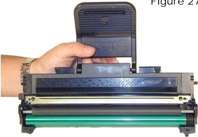
27) Fill the hopper with the appropriate toner. Replace the fill plug, check for leaks. See **Figure 28**
