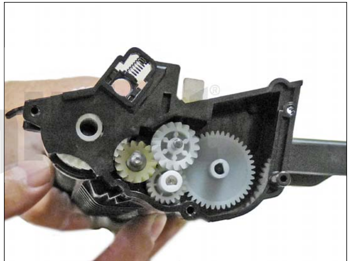
20. Install the four gears as shown.
