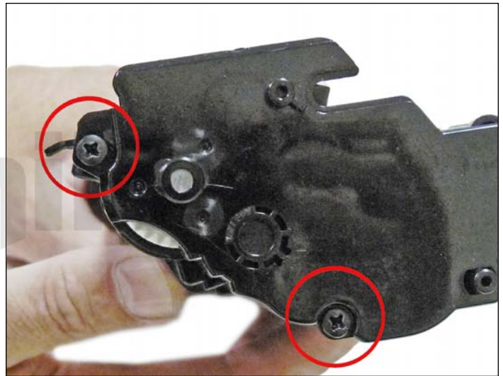
24. Install the gear side end cap, and two screws. Make sure the PCR fits correctly in its holder, and all the gears are aligned.
