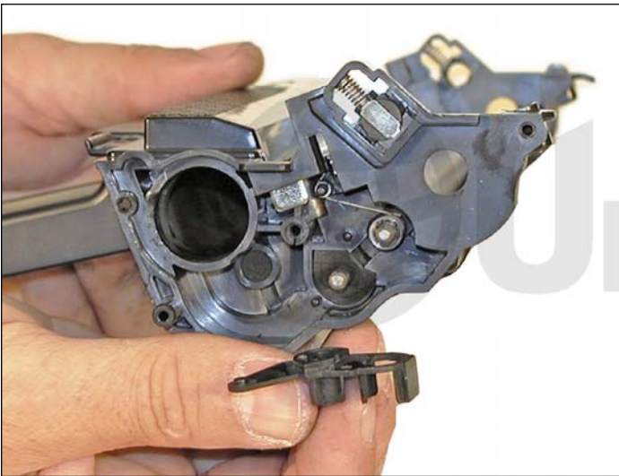
18. Install the roller plate.
