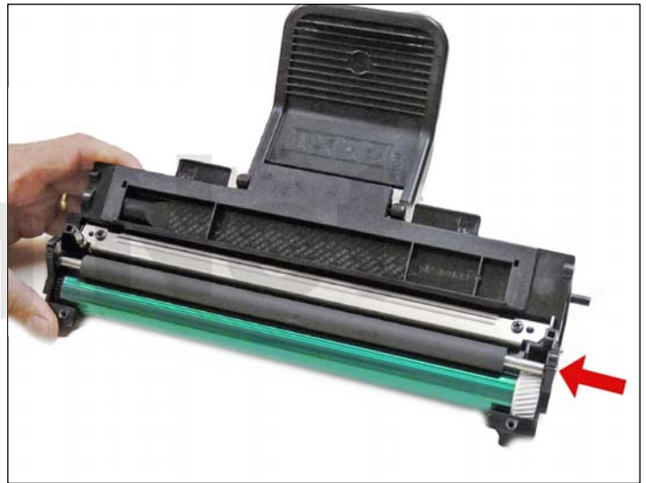
22. Install the PCR by sliding it through the large gear or non contact side, and into the contact hub.
