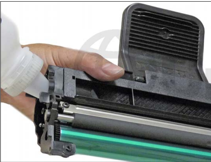
23. Fill the hopper with the appropriate toner. Replace the fill plug, check for leaks.
