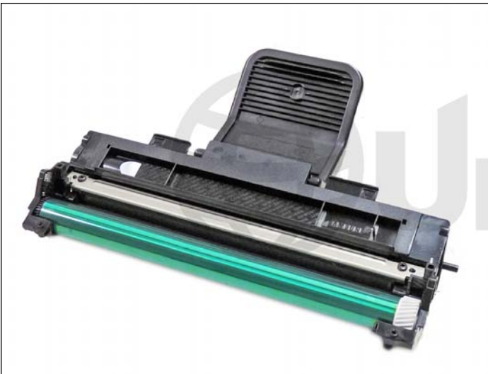
19. Install the drum in place.
