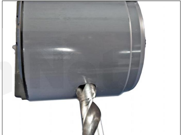
2. The hole can be drilled with a 1/2" drill bit or melted with a soldering iron. If it is drilled, great care must be taken to get all the shavings out. If it is melted, the outer edge of the hole has to be shaved flat with a razor blade. Clean out all the remaining toner/shavings thoroughly.
