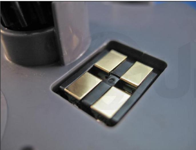
5. The OEM chip is not removed. A new chip is placed over it.
