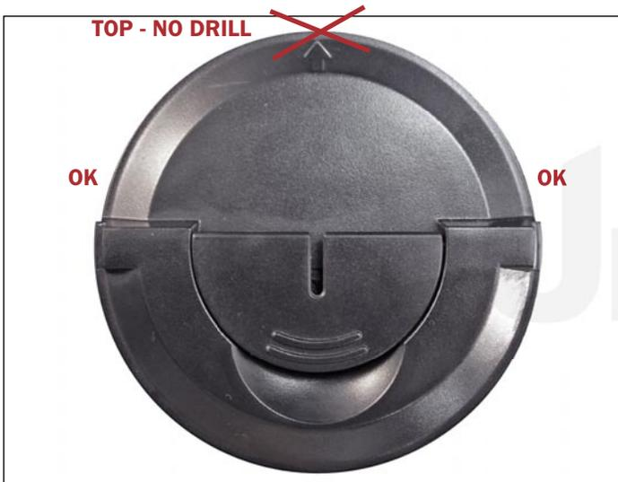
1. In order to clean and fill the cartridge, a hole must be drilled or melted into the cartridge. The hole cannot be placed at the top of the cartridge as that will cause cartridge problems.
