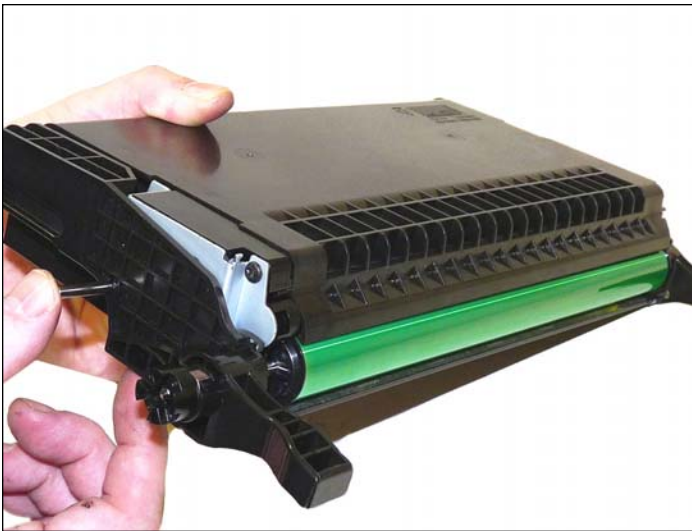
39. Install the two metal hinge pins.
