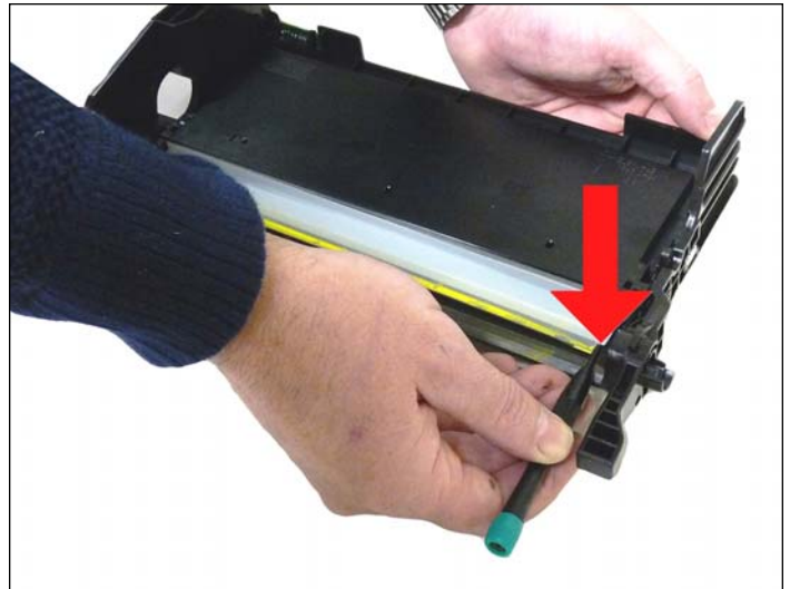
14. Remove the two screws and the wiper blade.
