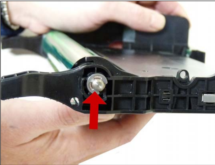
9. On the waste chamber, remove the E-ring from the non-drive gear side of the drum axle.
