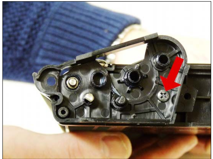
32. Install the inner gear plate and screw.
