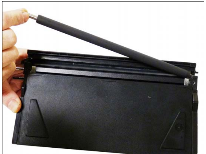
28. Remove the developer roller.
