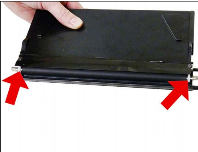
27. Remove the developer roller bushings.
