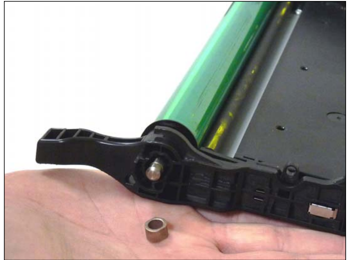
10. Remove the metal bushing.
