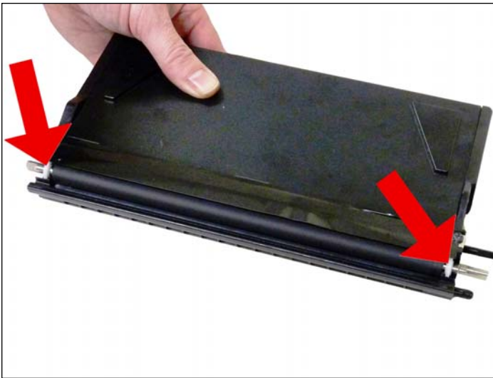
31. Install the developer roller and two bushings.
