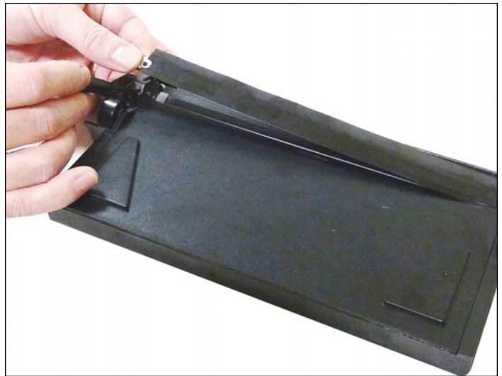
26. Carefully pry up on the doctor blade. The tape seal will come off with the doctor blade.
