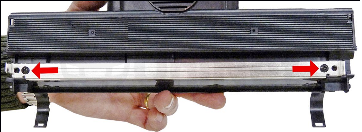
24. Remove the two screws from the doctor blade, and remove the blade.
