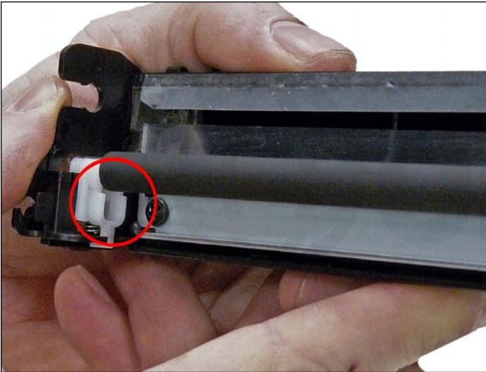
19. Place a small amount of conductive grease in the PCR holders, and install the PCR. Note that there is a spot on the holders for a PCR cleaning roller. They are not used in the cartridge.
