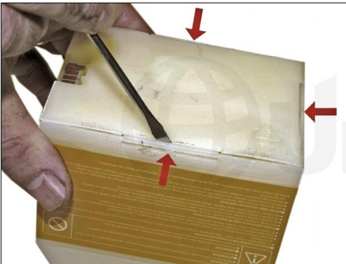
1. Open the tabs on the top cover (side that holds the chip, opposite of the feed valve) of the cartridge by releasing the interlocking clips. There are three clips, one on each side minus the chip side.
