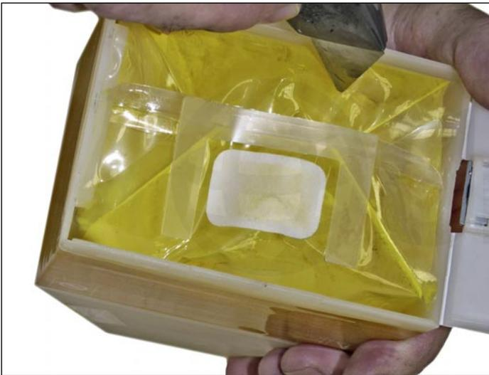
3. Cut a small incision on the plastic bag that will allow you to clean out the old toner and to fill it again. This slit will be sealed with tape when done.
