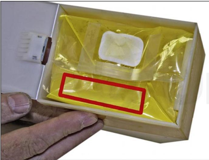
5. Clean the outside of the bag as much as possible and seal the slit closed with a good packing tape.
