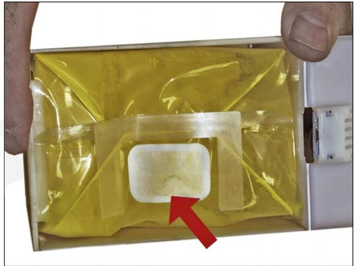
2. Once you release the clips, the cover can be lifted revealing the toner bag.
