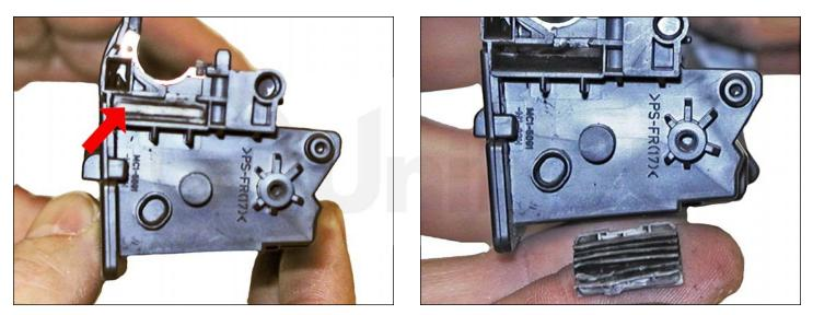
19. When a seal becomes available, remove the seal port plug, and install the seal. Bring the tail out through the seal porthole. Install the plug.
