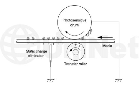
In the **fourth step** (Transfer Block) the toner image is then transferred to the paper as it passes below the drum by the transfer charge roller, which places a positive charge on the back of the paper. This positive charge causes the negatively charged toner on the drum's surface to be attracted to the page. The small diameter of the drum, combined with the stiffness of the paper causes the paper to peel away from the drum.
