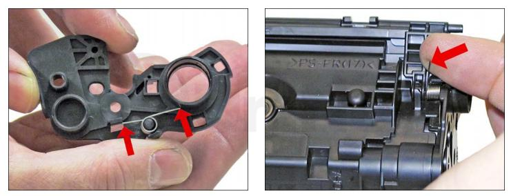
27. With the drum cover spring as shown on the end cap, install the end cap.
