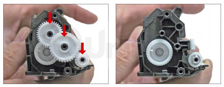
13. Remove the gears from the hopper as shown.
