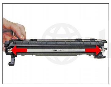
21. Install the doctor blade and two screws.
