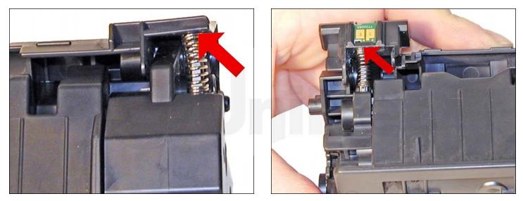
26. Set the hopper tension springs back in place.
