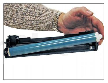
11. Install the new/cleaned drum hub side first.
