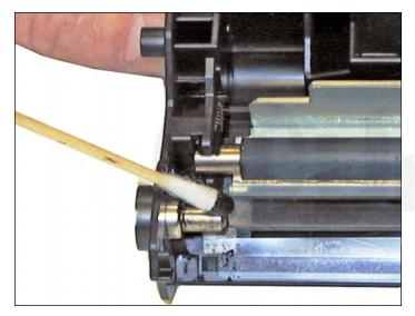
10. Place another small amount of conductive grease on to the metal drum axle.
