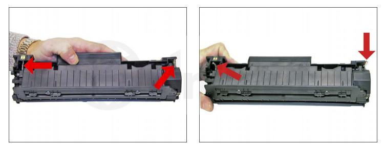
2. With the pair of needle nose pliers, release both the hopper tension springs.
