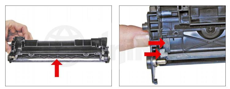
7. Clean out all the waste toner from the hopper. Be careful not to damage the recovery blade located next to the wiper blade.
