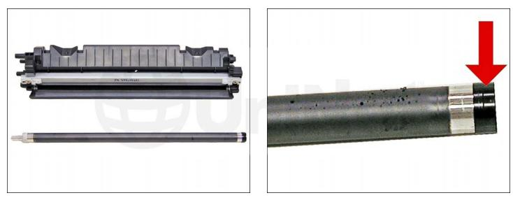
15. Remove the magnetic roller assembly.
