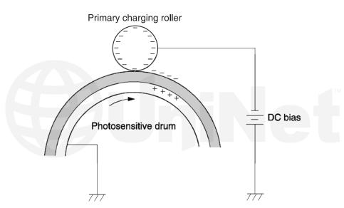
The image formation process consists of a series of steps. In the **first step**, the Primary Charge Roller (PCR) places a uniform negative DC Bias voltage on the OPC drum surface. The amount of the negative DC Bias placed on the drum is controlled by the printer intensity setting. This process is part of the Latent Image Formation Block.
