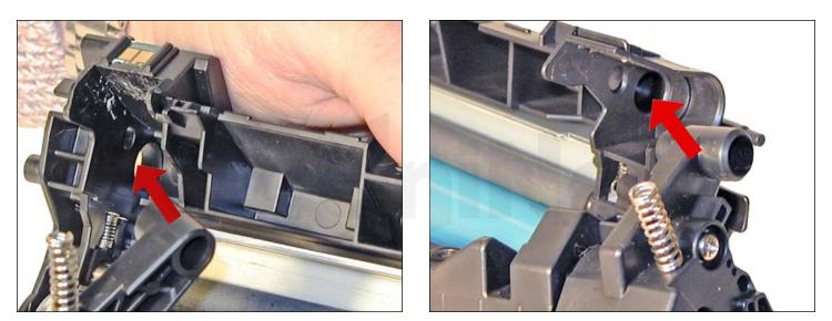
25. Place the drum/waste hopper into the toner hopper.Slide it over so the round hinge pins fit into their respective holes.
