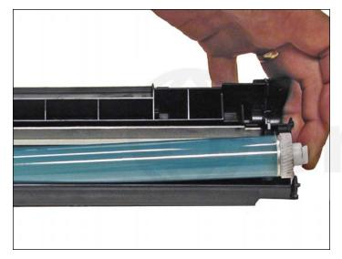
4. On the waste/drum section, lift the drum up from the gear side. Twist and remove from the hopper.
