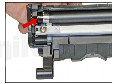
22. Install the magnetic roller black bushing side first. Turn the roller until the keyed end locks in place.
