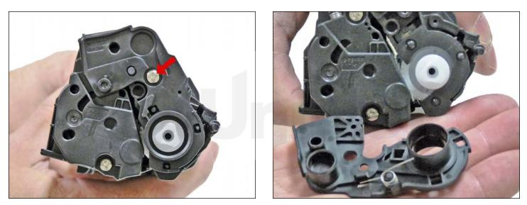
1. With the handle facing you, remove the right side screw and end cap from the cartridge.
