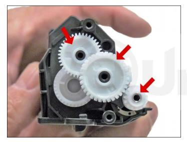
23. Install the gears as shown.
