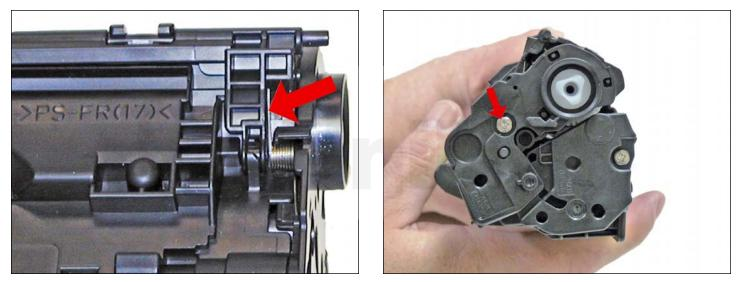
28. Lift up the drum cover spring tail to fit as shown on the drum cover.
