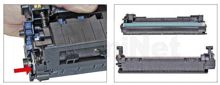
3. Slide the waste/drum section over to the left side.
