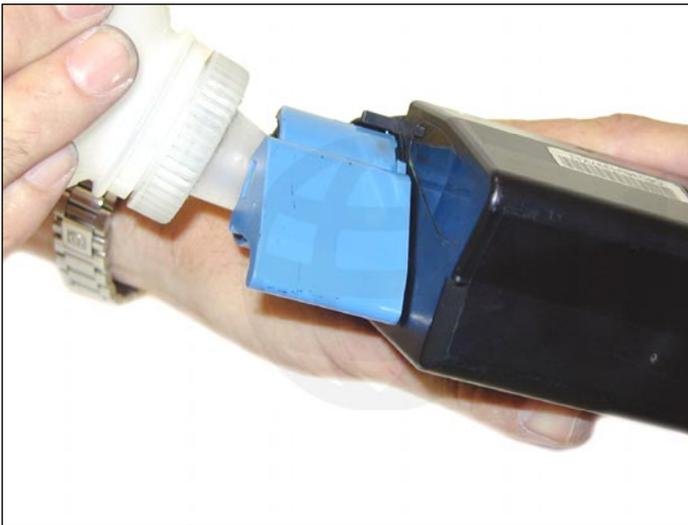
4. Close the port, fill with new toner, and replace the fill plug.
