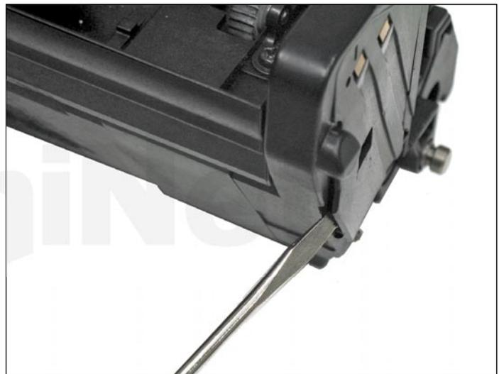
31. We will need to insure that the reflective target is clean. To do so, remove the cover found in the smaller end cap as shown.
