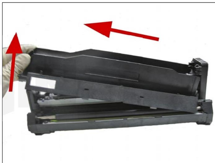
14. Remove the top cover, lifting the left side first and pulling away from the cartridge as shown.
