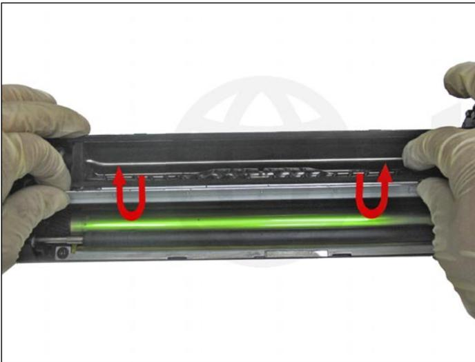
16. Remove the doctor blade by flipping it 90 degrees to clear the metal extension as shown.
