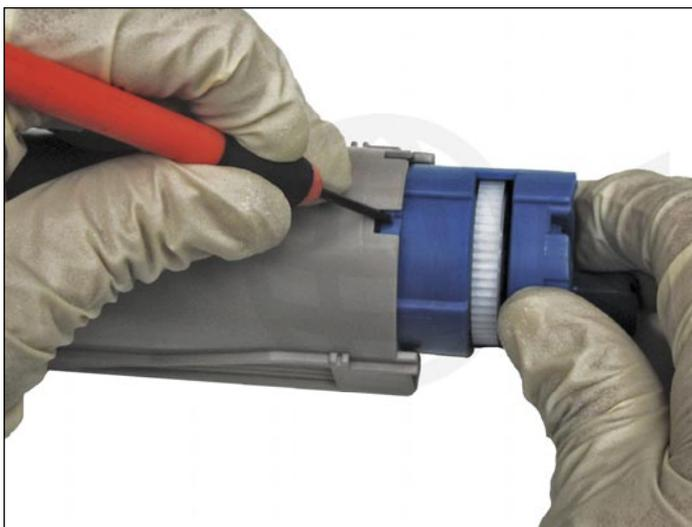
3. Push down the locking tab while you rotate the blue handle, which will make it easier to remove the rest of the blue portion.
