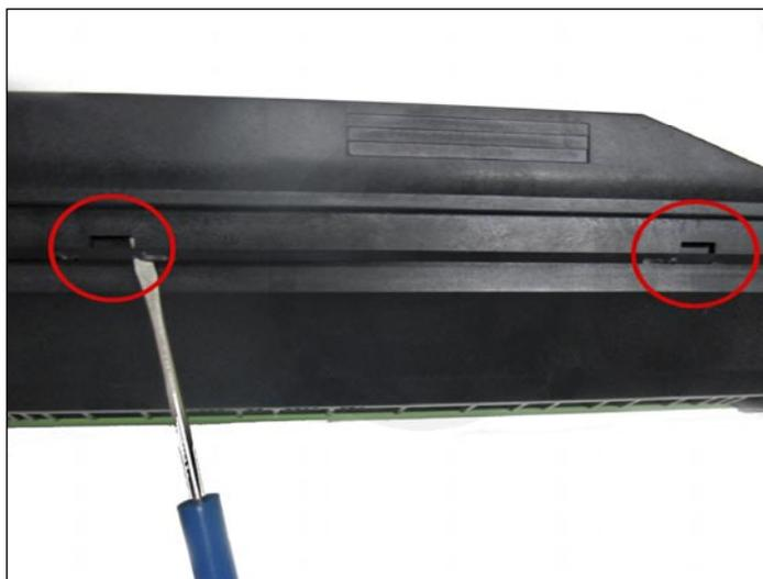
13. Turn the drum unit over so the bottom is facing up. Release the locking tabs by pressing them in using a flat screwdriver.
