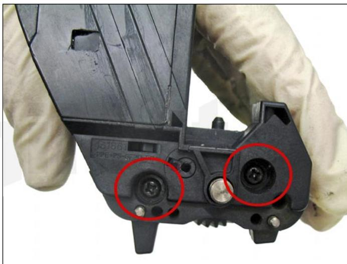
21. Remove the two screws from the smaller end cap on the opposite side.
