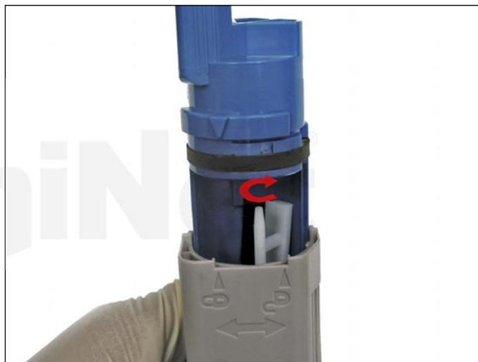
9. **NOTE:** To easily install the blue handle, rotate the actuator until it is centered. This may require several turns and adjustments to center it. Once centered, insert the blue handle as shown.
