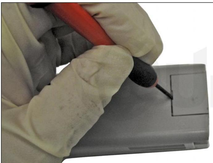
10. Locate the chip compartment on the top side of the cartridge opposite of the blue handle. Using a small, flat head screwdriver, pry off the cover.
