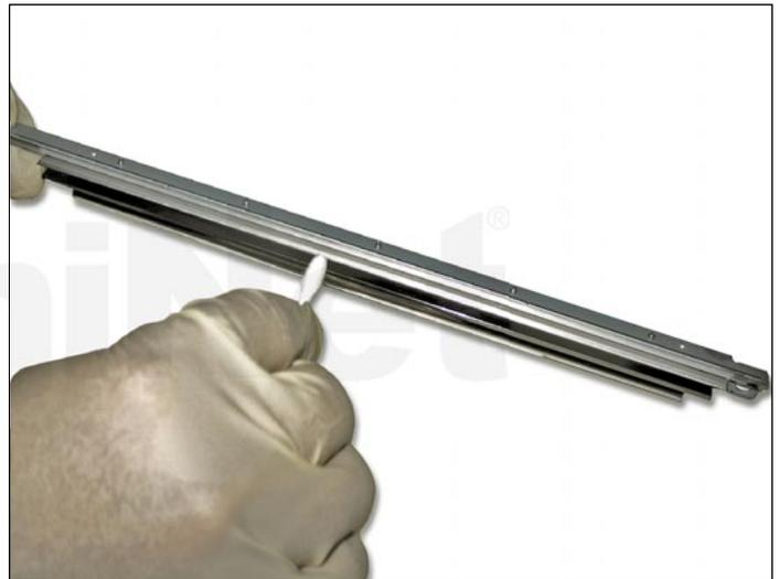
17. Clean the edge of the doctor blade using a cotton swab with 99% isopropyl alcohol first, then purified water. This will remove any residual toner.
