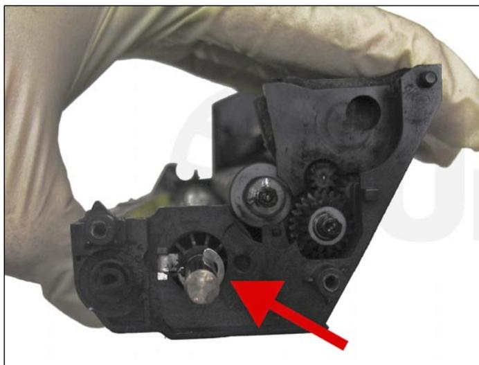
20. Remove the C-clip to unlock the drum axle shown.
