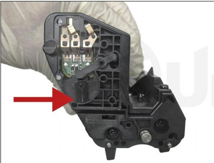
32. Clean the shown target using a small cloth with isopropyl alcohol and install the cover.
