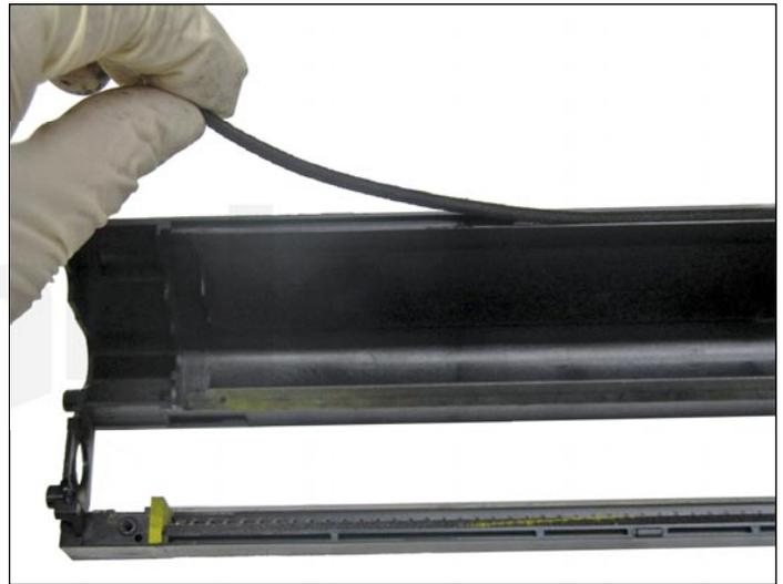
26. Finally, remove the supply roller assembly and clean the cartridge thoroughly.
