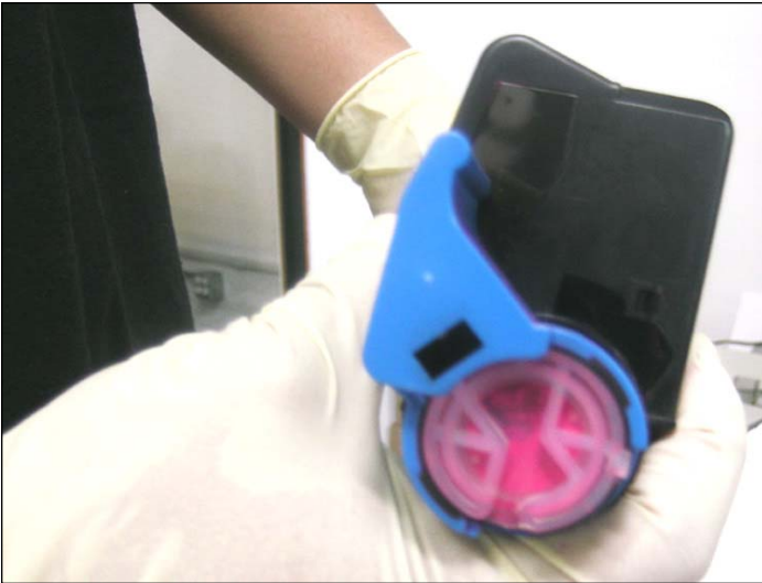
35. White tab lifted. Remanufacturing concluded.
