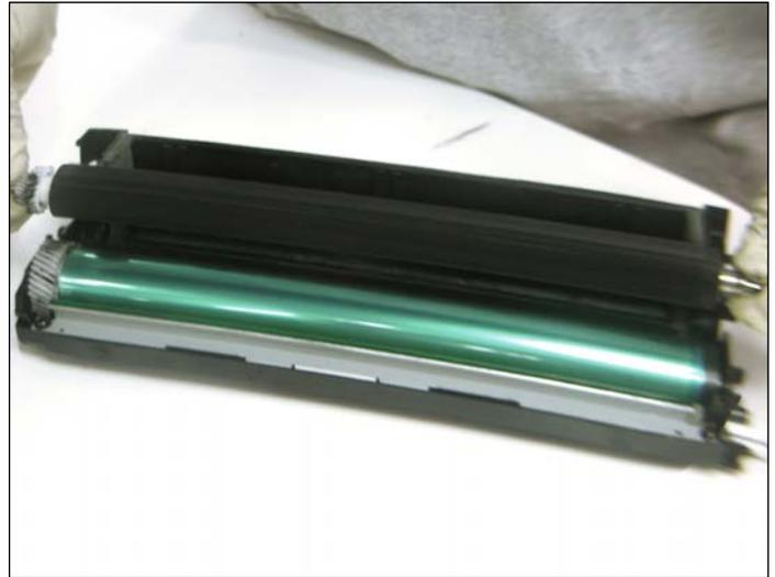
15. Remove the developer roller as shown.
