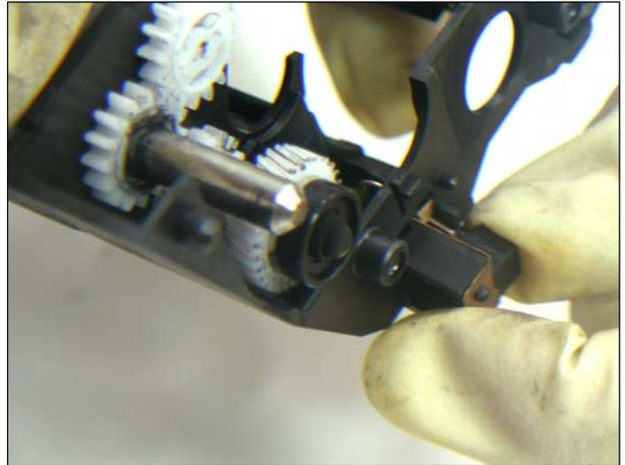
19. Pull out the fuse holder located on the side of the cartridge.
