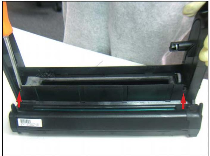
4. Remove the two screws located on the the top of the drum unit cover that hold it in place.
