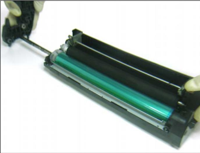
12. Slide the end cap with axle out completely.
