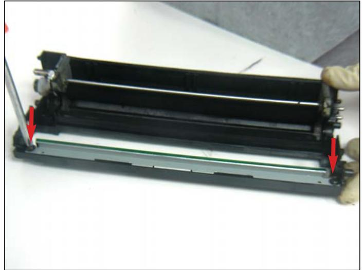
17. Remove the two screws on both ends of the wiper blade that hold it in place.
