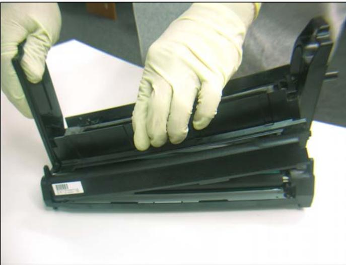
6. Remove the drum unit cover as shown.
