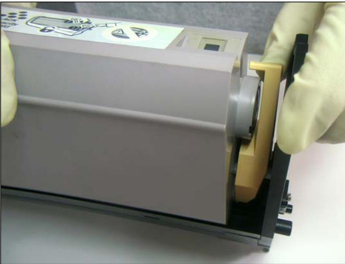
1. Release the toner hopper from the drum unit by turning the yellow handle down from its upright “locked” position as shown.
