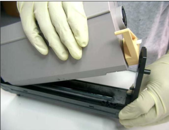
3. Lift the hopper from the drum unit, starting from the blue handle side as shown, then set aside.
