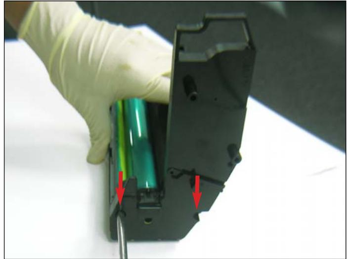
13. Remove the screws on the remaining end cap (gearside) that hold it in place.
