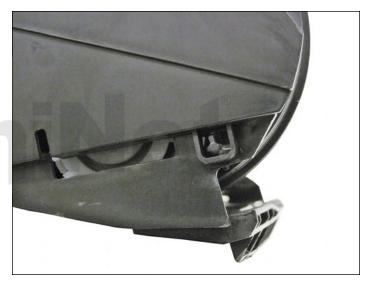
5. Slide the left side of the OEM toner hopper into the universal conversion cover. Make sure that the white wheel slides under the retaining hook of the conversion cover and that the shipping lock peg of the OEM toner hopper fits into the hole on the conversion cover.
