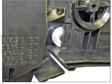
6. On the opposite side of the conversion cover, pull the right side wall out with one hand and use your other hand to snap the OEM hopper in place until the white wheel clicks and locks under the retaining hook. On the backside, make sure the shipping lock peg fits into the hole on the conversion cover.
