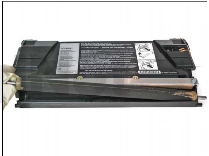
9. Remove the developer roller.
