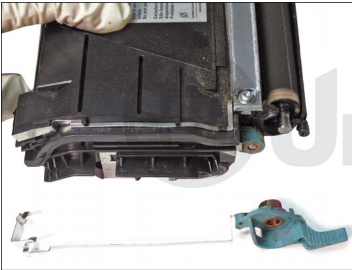
8. Remove the support plate along with its rear contact.
