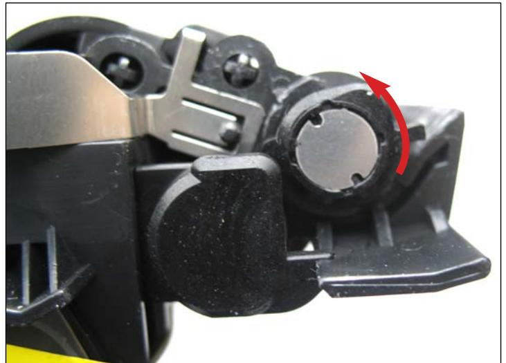
8. Rotate the developer roller support counter-clockwise to release it.
