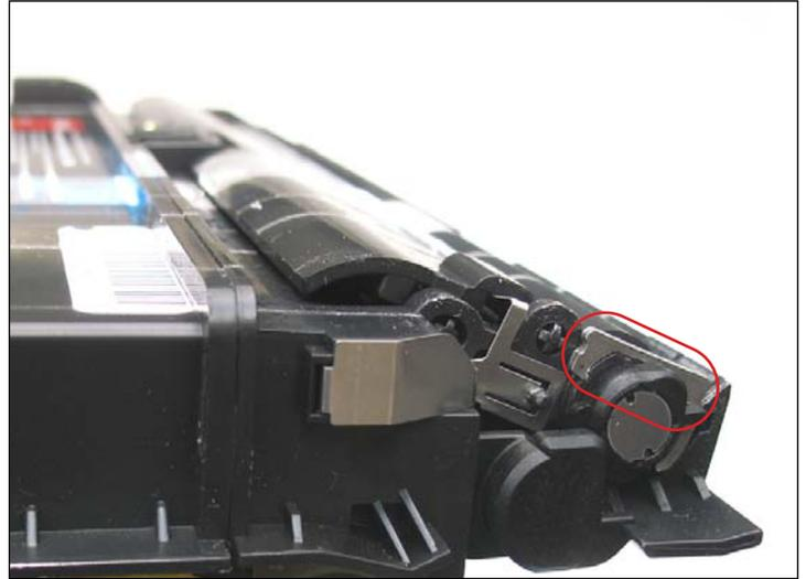
6. Contact-side of the cartridge with security bar (highlighted).
