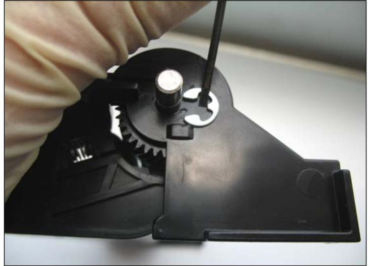
14. Using a small flat screwdriver, remove the drum axle "C" clip from both ends .
