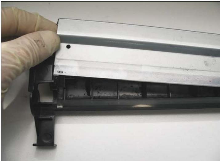
19. Remove and clean wiper blade using a lint-free cloth.
