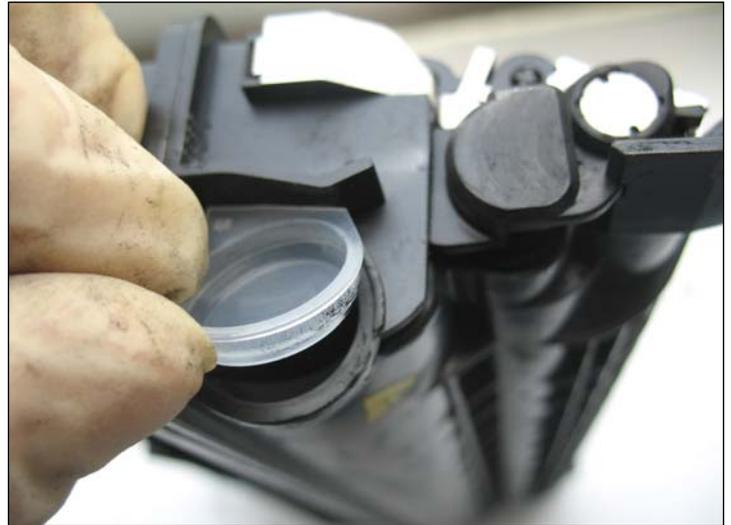
12. Remove fill plug and clean cartridge thoroughly. Once clean, reassemble and refill.
