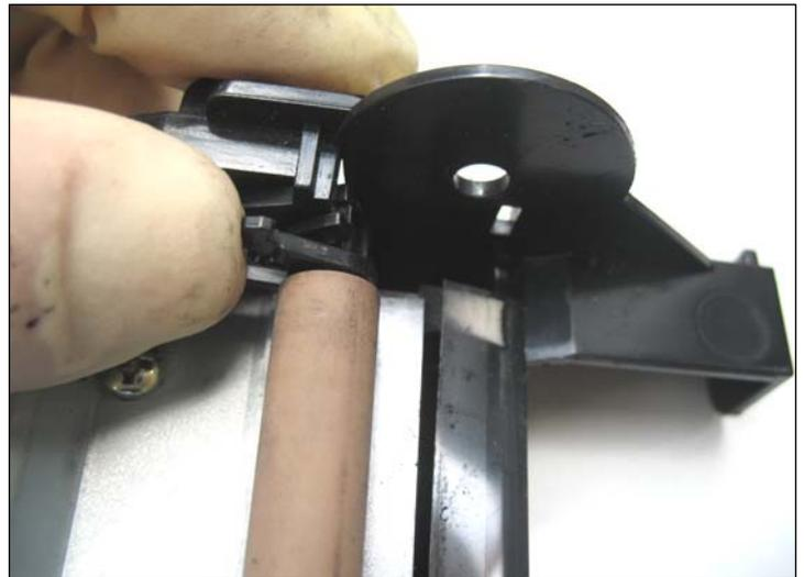
16. Unlock the PCR by pushing out the lateral tabs.
