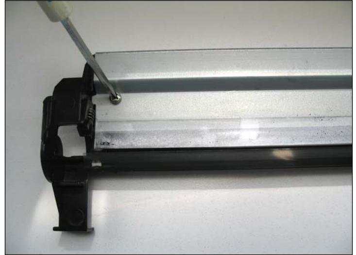
18. Remove the screws from each side of the wiper blade.
