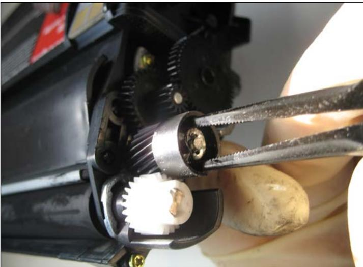
3. Using needle-nose pliers, release the idle gear (shown) by removing the locking clip that holds it in place.
