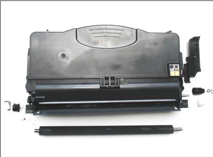
11. Toner cartridge disassembled.
