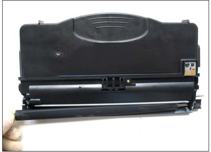
10. Pull the developer roller out from the contact-side of the cartridge.
