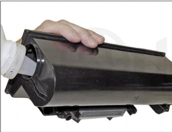
3. Fill the cartridge with toner for use in the TK-60 series of cartridges. Replace the fill plug.
