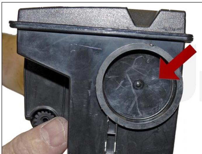
1. Remove the fill plug from the cartridge.
