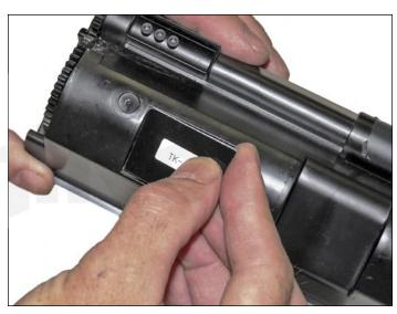
4. Peel off the old chip label (it is an RF type chip).
