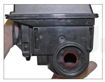
1. Drill a 1/2" to 3/4" hole into the fill plug. The OEM plugs are welded in so the hole is necessary. Clean out all the remaining toner.
