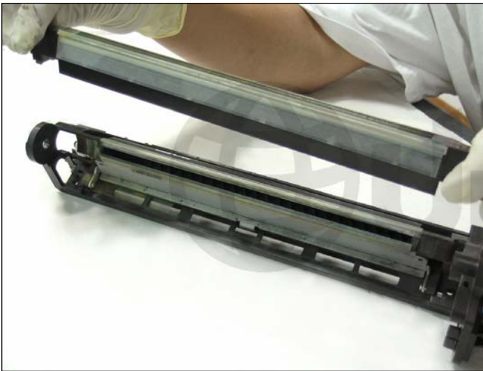
6. Remove the primary charge unit as shown.
