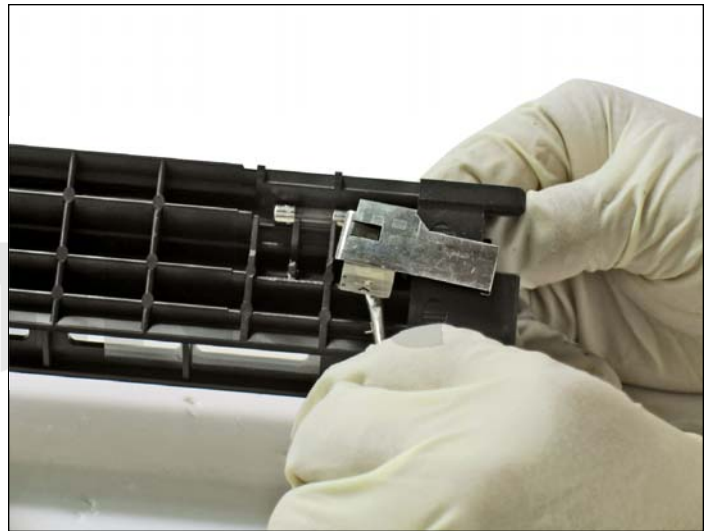
11. Pull out both metal plates shown using a flathead screwdriver.
