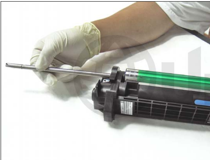
3. Carefully pull out the axle from the opposite end.
