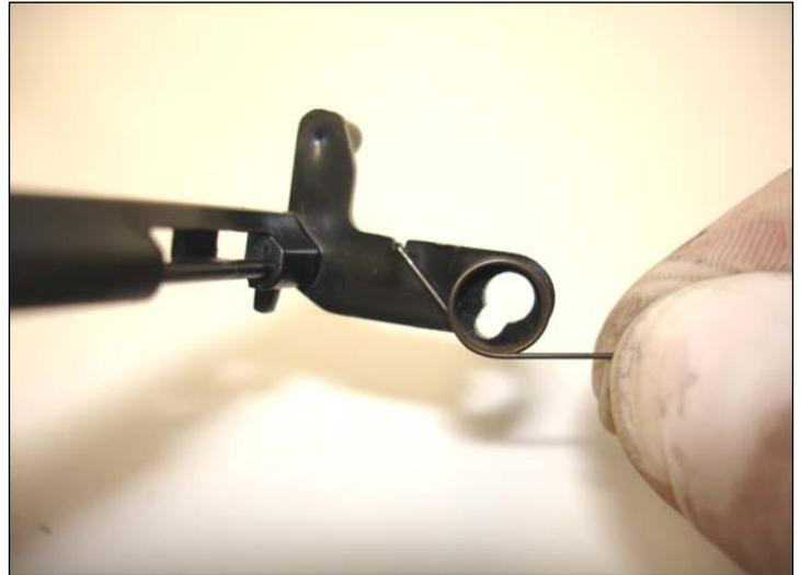
28. Place the spring as shown in the drum shutter arm.
