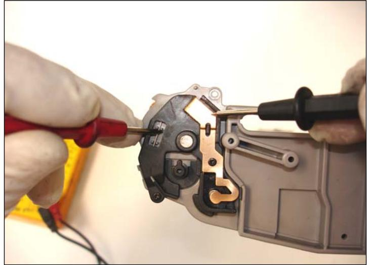
26. Check the electrical continuity with a tester to ensure good contact between both parts of the contact end plate.
