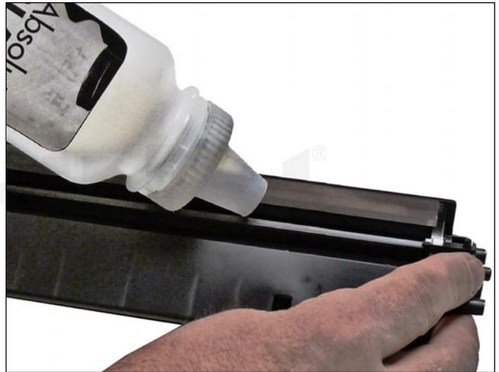
19. Fill the hopper with new replacement toner for use in the HP Pro M125.
