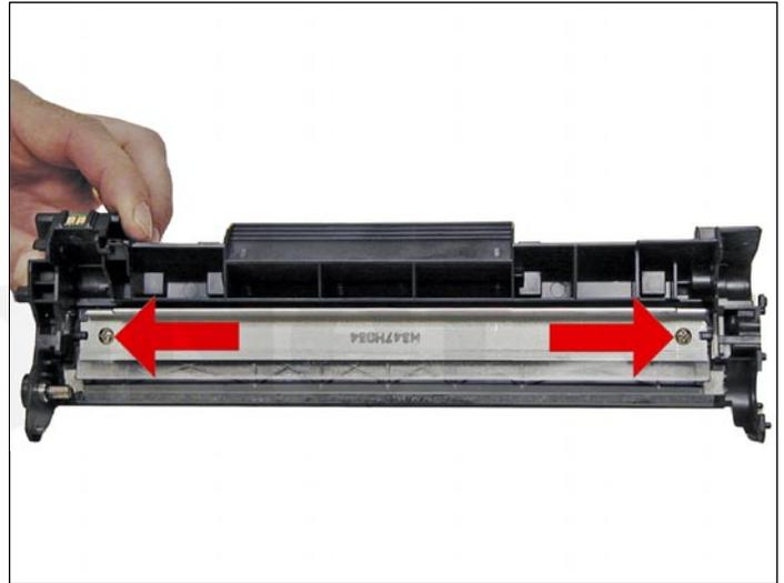
6. Remove the two screws and the wiper blade.
