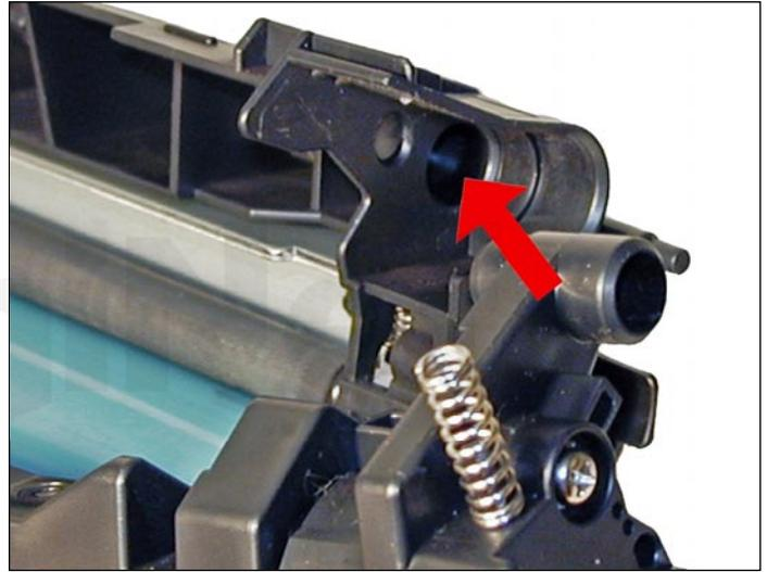
26. Place the drum/waste hopper into the toner hopper.
