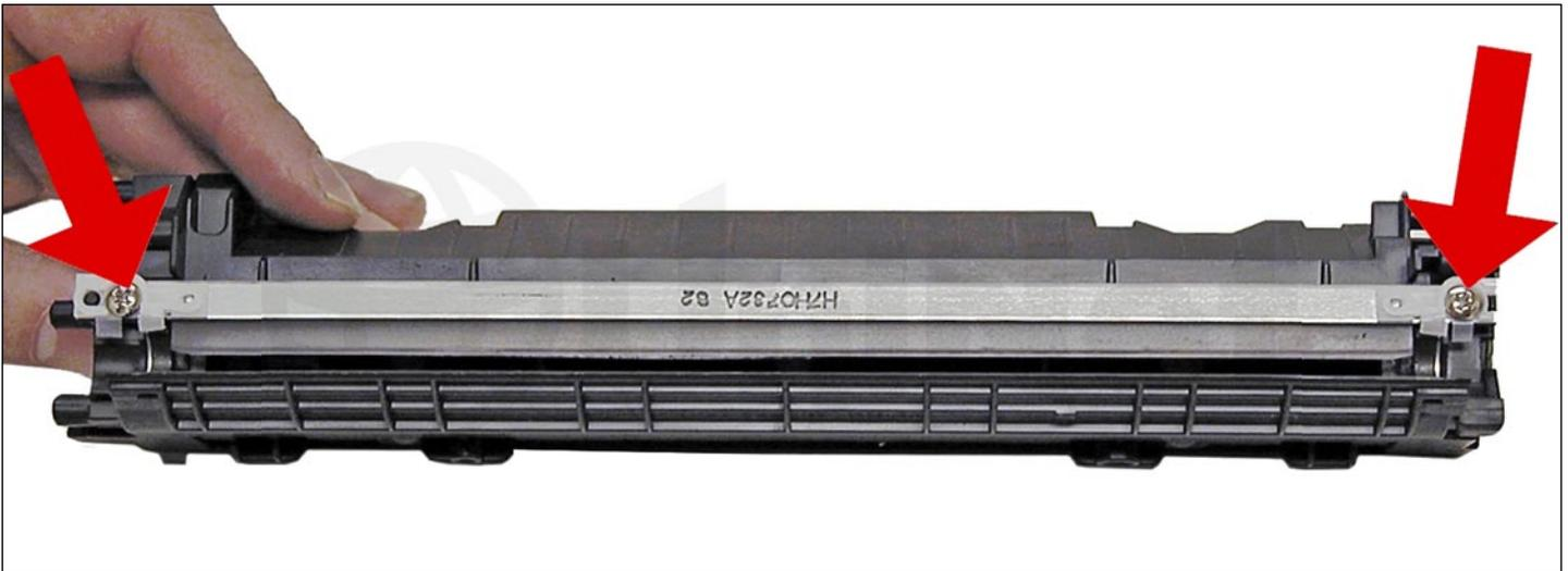
17. Remove the doctor blade and two screws.
