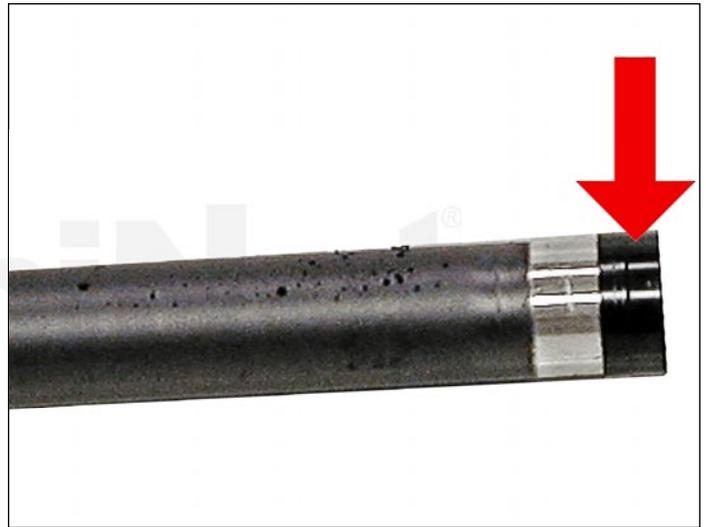
16. Remove the magnetic roller assembly.
