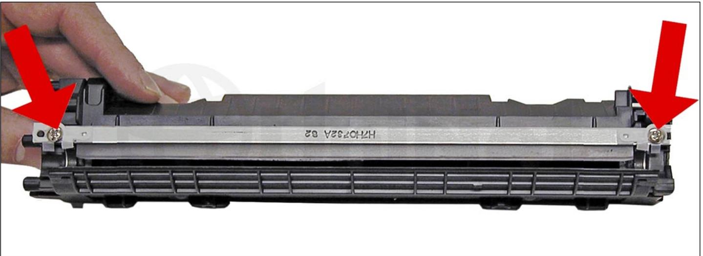
22. Install the doctor blade and two screws.
