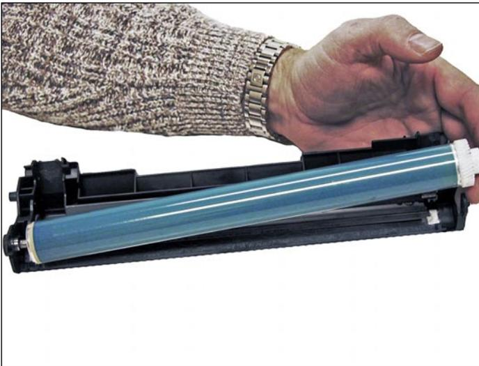
11. Install the new/cleaned drum, hub-side first.
