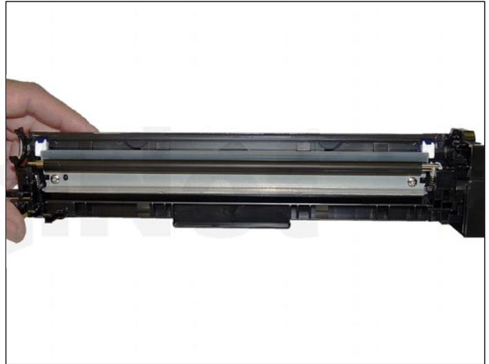
11. Install the cleaned PCR.
