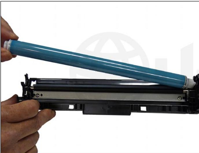
6. Remove the drum from the waste chamber.
