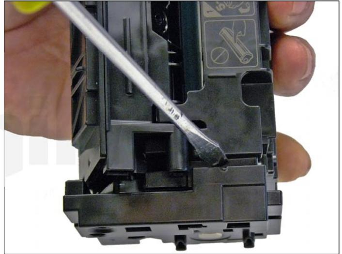
2. On the same side, using a flat blade screwdriver, pry out the top of the end cap until you feel the weld give way.
