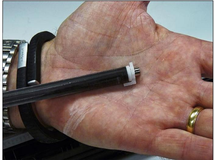
16. Slide the developer roller over and remove.
