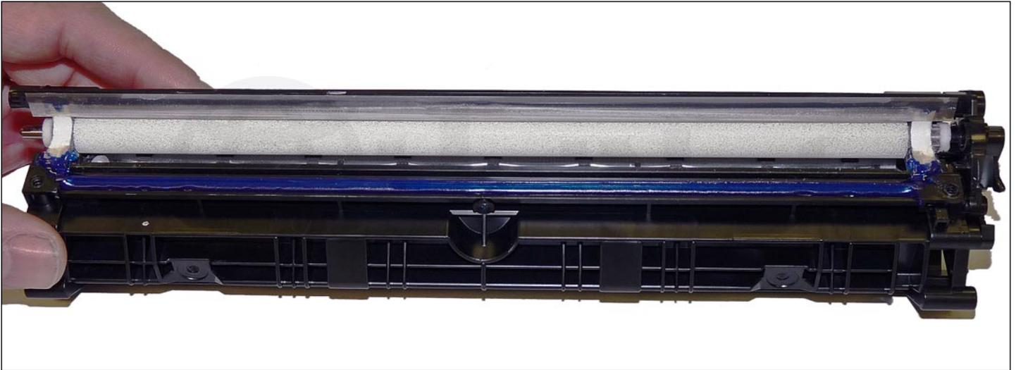
18. Vacuum out the remaining toner from the hopper from the slot next to the feed roller.
