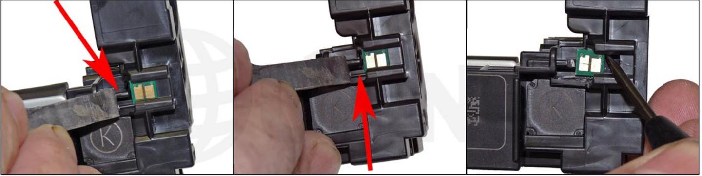
27. Cut the chip holder with a flat blade in the two places indicated.
