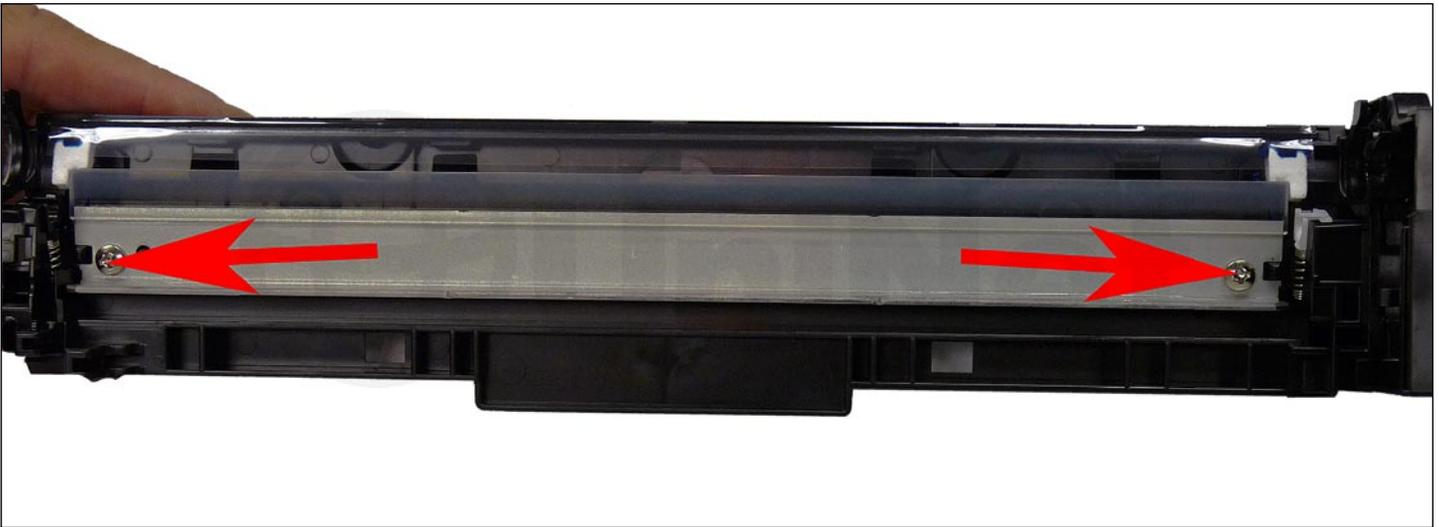
10. Coat the new wiper blade with your preferred lubricant and install.
