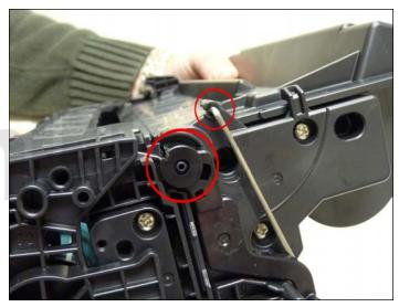
32. Install the spring in the drum cover arm as shown.
