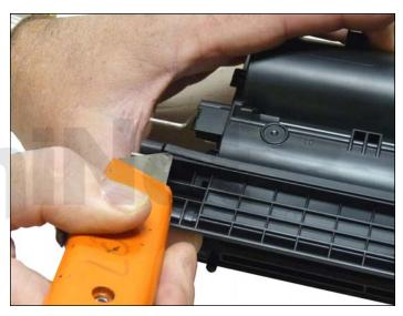
20. If you want to seal the cartridge, the hopper must be split. This can be done with a sturdy razor knife and screwdriver. Take the knife and split the hopper along the seam.
