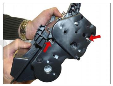
29. Install the gear end cap and two screws. If the end cap does not fit, the stationary magnet most likely is not set correctly. The end cap has deep holes. Using a magnetized screwdriver will make your life much easier.
