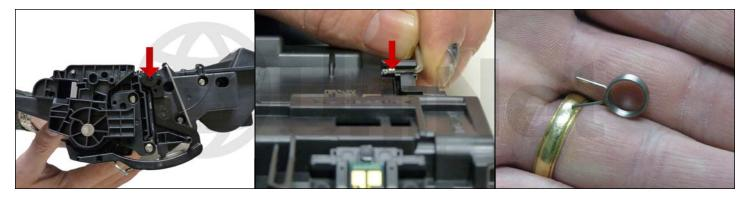
1. Remove the drum cover by prying the spring loaded arm, and then carefully pry off the two metal bars out of their holders.
