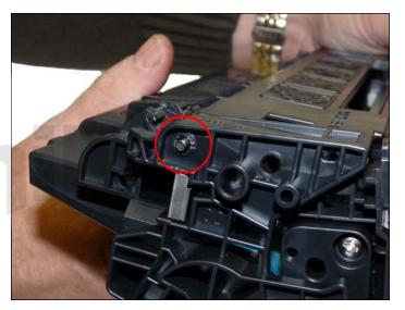
31. Place the two halves together. Make sure the springs are set, and install the two pins. The pins should not be pushed in until they are flush with the cartridge wall. Install them so they match what the OEM did. They should protrude about 1/16" from the flat wall so you can easily remove them again.
