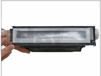
23. Place the seal on the bottom hopper, and rail foams on the top half of the hopper. Make sure you place the tail of the seal over the correct side (opposite the gear).
