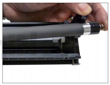
17. Remove the magnetic roller assembly from the cartridge.
