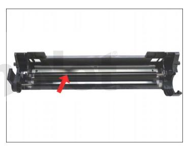
6. Remove the primary charge roller (PCR), by prying it out of the clips on either end. Clean the PCR with your preferred cleaner and place the aside.
