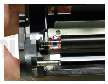
10. Clean the two PCR holders and place a small amount of conductive grease on the black PCR holder, and a small amount of white lithium grease on the white holder. Install the cleaned PCR. Note the colored band on the OEM PCR. It looks like Canon/HP are color coding production lots.
