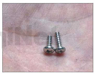
18. Remove the two screws and doctor blade. Keep these screws separate! They are longer than all the other screws used in this cartridge. Clean out any remaining toner. **NOTE**: The cartridge can be filled now of the hopper split, filled and sealed.
