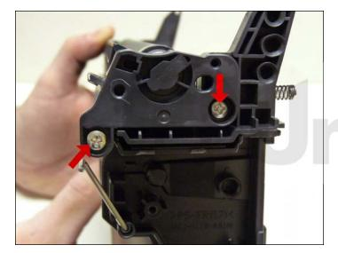
16. Remove the two screws and the magnetic roller end cap.
