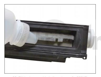
22. Fill the hopper with dedicated toner for P3015:295g for the "A" cartridge and 590g for the "X" cartridge.
