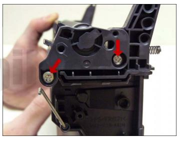
27. On the non-gear side, install the magnetic contact end cap and two screws. Clean the magnetic roller sleeve with a dedicated magnetic roller cleaner.
