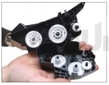
14. Remove the end cap. Note that three of the gears stay with it. Leave the remaining two large gears alone. They drive the mixing augers and are very hard to replace properly if removed.
