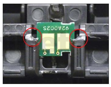
34. To replace the chip, cut the melted plastic from the top edge of the chip.
