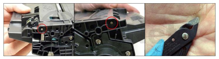
2. Note on each end of the cartridge there are small silver pins. Unlike most cartridges these days, the pins are easily accessible from the outside of the cartridge. Use a good pair of flush cutting wire cutters to pull the pins out. The image above on the far right shows what flush cutting wire cutters look like (the blades meet with a flat surface, not curved in like most cutters).
