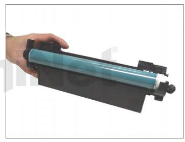
11. Clean and replace the conductive grease on the drum axle pin.
