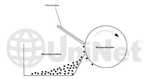
In the **seventh step** (drum cleaning block) the OPC drum is cleaned. On average, approximately 95% of the toner is transferred to the paper during the print cycle. As the drum rotates during printing, the remaining 5% of the toner that is on the OPC drum is cleaned off the drum by the wiper blade. It is then guided into the waste chamber by the recovery blade, and stored in the waste chamber.
