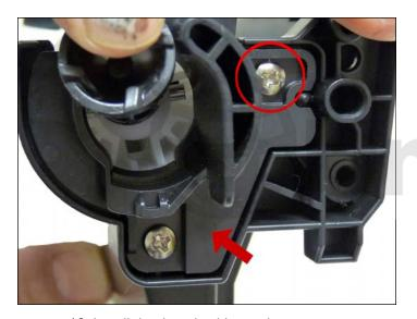
12. Install the drum bushing and two screws.
