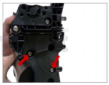
15. On the contact side, remove the two screws and end cap.
