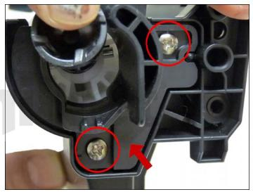
4. On the waste section, remove the two screws and drum bushing.
