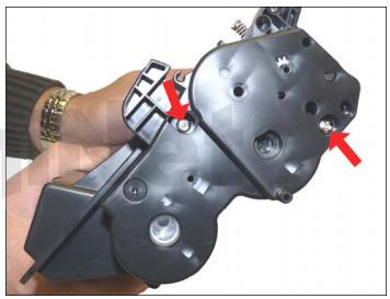
13. On the supply section, remove the two screws from the right side (gear side) end cap.
