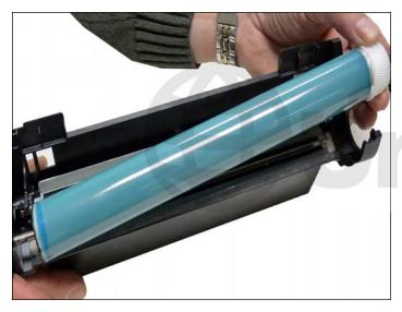
5. Remove the photoconductive drum. Pull it gently from the drum axle pin. The pin can be removed to make removing and installing the drum easier, but the plastic is a bit soft and if not installed back perfectly, the drum axle hole will be enlarged allowing the drum to float.
