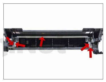
8. Clean out any remaining waste toner. Make sure the foam seals under the wiper blade are clean and not damaged.
