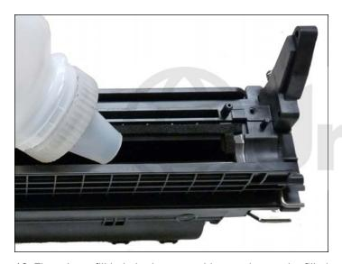
19. There is no fill hole in these cartridges so it must be filled through the doctor blade slot. Fill the cartridge with 295g for the "A" cartridge and 590g for the "X" cartridge of dedicated toner for P3015. **Skip to step 25.**
