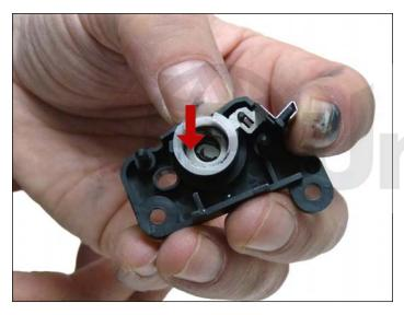
26. Clean the magnetic roller contact plate on the contact end cap. Replace the conductive grease.
