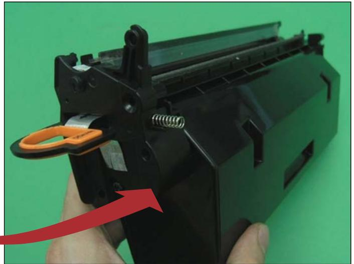
14. Now install the left end cap onto the left side of the hopper. The P2015 left end cap includes the pull tab feature like the OEM, but does not include the orange clip. The orange clip is available separately or you can use the OEM orange clip.
