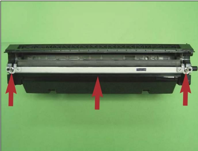
11. Install the doctor blade into the hopper and place the mag roller wiper on each end of the doctor blade. Tighten the two screws that hold the doctor blade and wipers in place.
