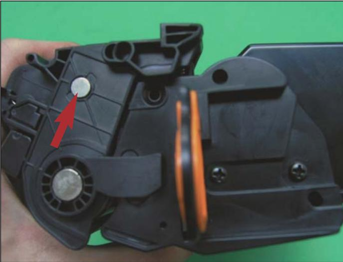
17. Assemble the Hopper side and Waste Hopper together and insert the hinge pin on each side to hold them together.
