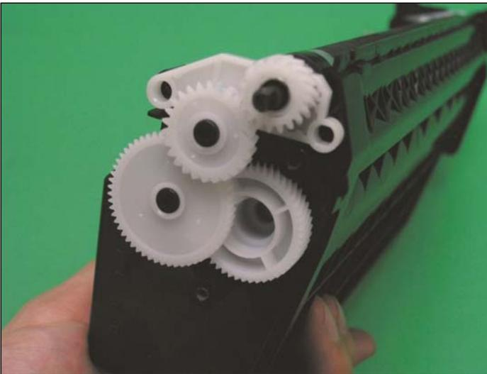
15. Install the mag roller in the hopper as shown in the photo. Then insert the right stabilizer, and all drive gears on the right side of the hopper.
