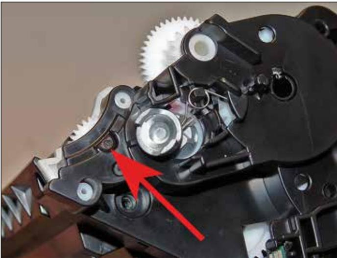
34. Install the gear end cap and three screws. You might have to turn the magnetic roller shaft slightly for the end cap to fit properly the end is keyed and fits into a keyed slot in the end cap.
