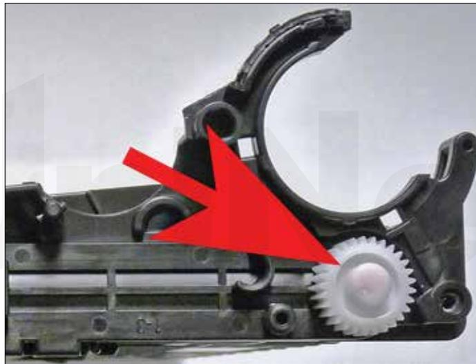
13. Snap the auger cover back in place and install the two screws.
