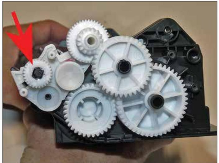
33. Install the magnetic roller drive gear.
