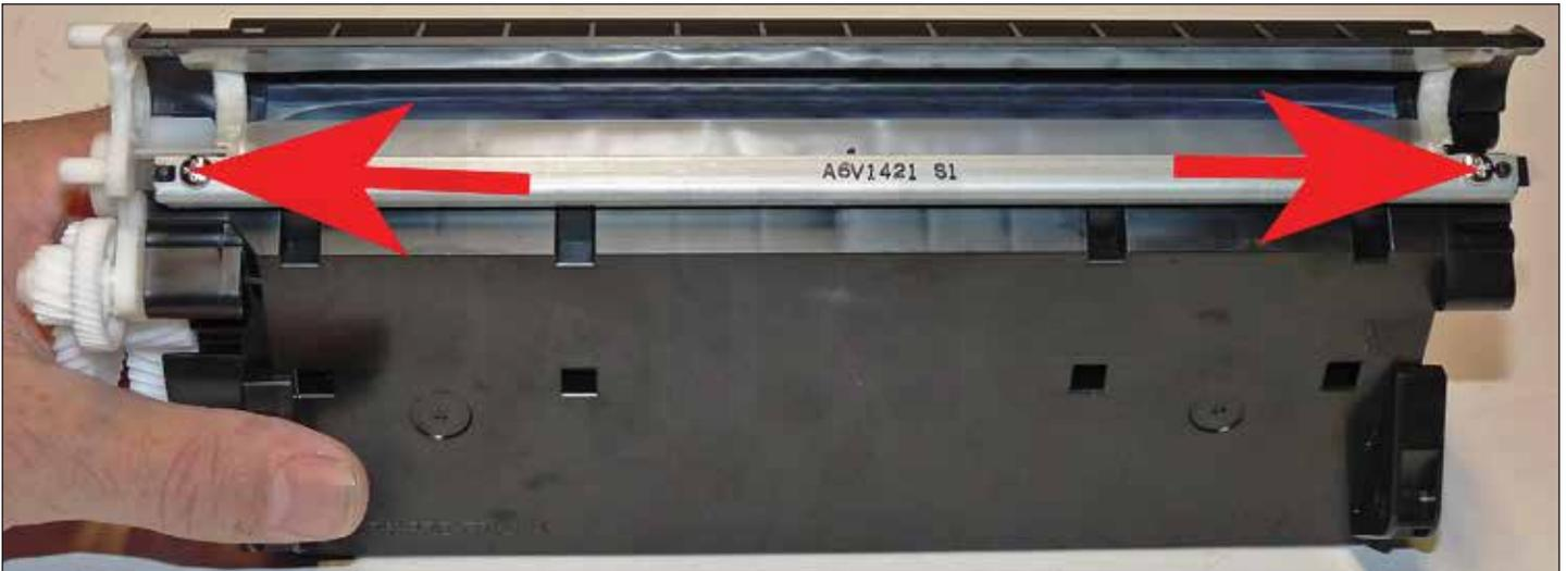
30. Install the doctor blade and two screws.
