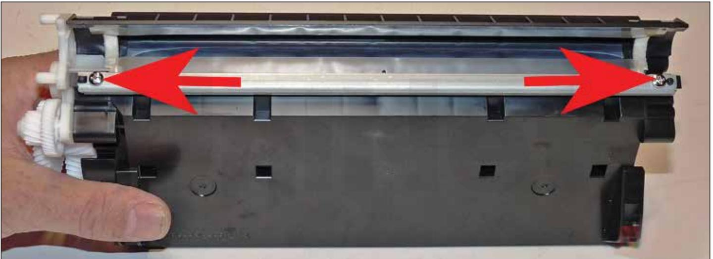
28. Remove the two screws from the doctor blade.
