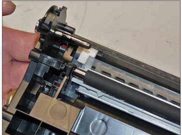
18. Clean and replace the conductive grease on the drum axle.
