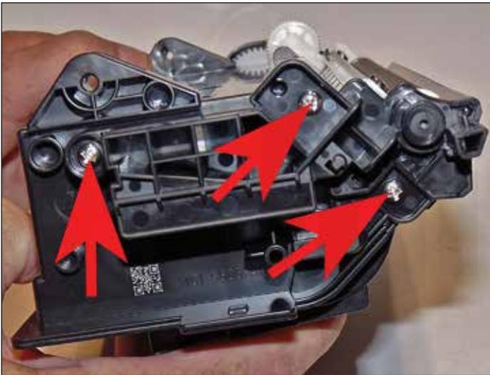
32. Install the white bearing on the magnetic roller, the non-gear end cap and three screws.
