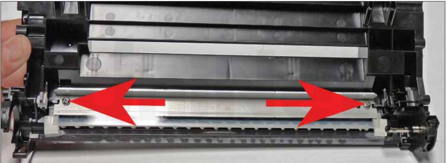
15. Install a new or cleaned, lubricated wiper blade and two screws.
