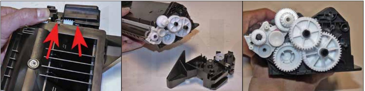
25. Press in on the two bottom tabs and pry off the end cap.
