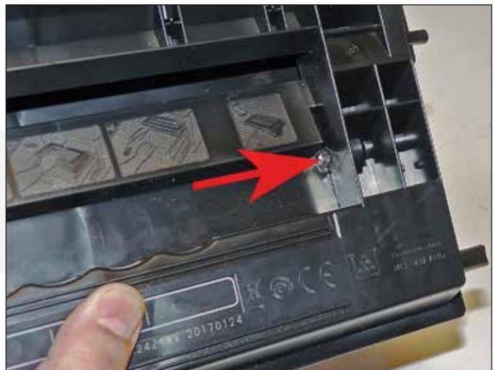
2. Drill a small hole in the top of each side of the cartridge as shown.
