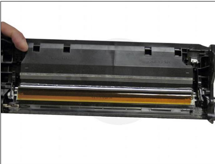
15. The amber film assembly is held in place with double-sided tape. If this is not adhering, or a new wiper blade is being used, replace the tape. Replace the film assembly.
