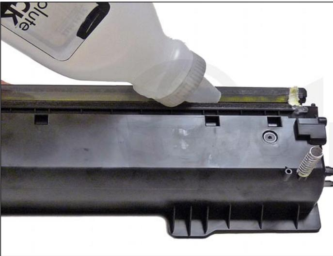
33. Clean out the remaining toner and fill with the correct color of toner for use in the M651/M680 series.
