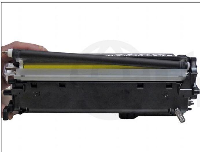
41. Install the cleaned developer roller. Do NOT use any chemicals to clean this. A lint free cloth works fine.
