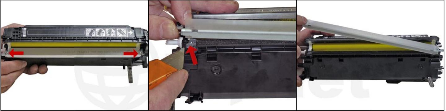
28. Remove the two screws from the doctor blade and start to lift the blade up.
