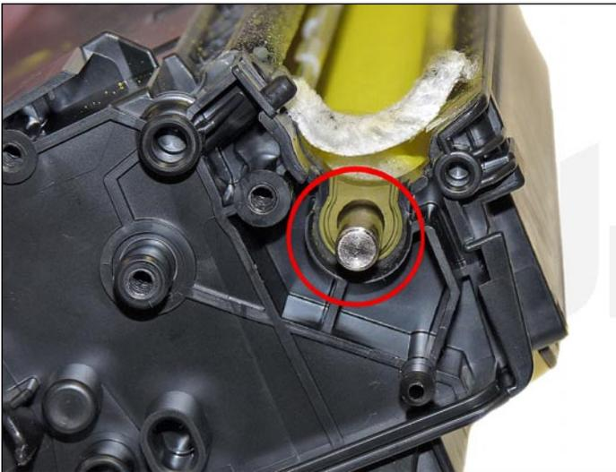
36. Install the feed roller and rubber bushing.
