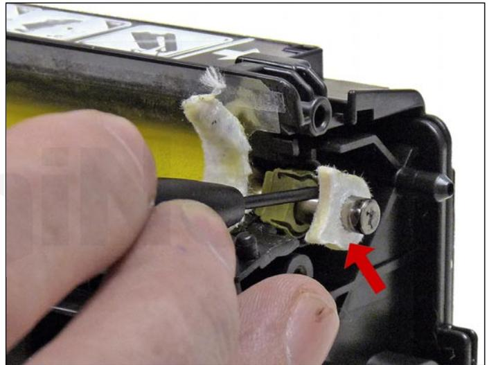
30. Remove the white felt washers from both sides of the feed roller.
