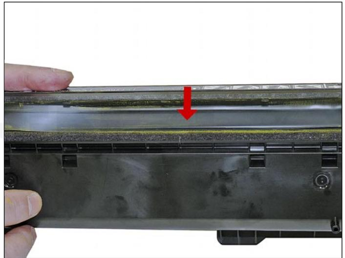
34. When a seal is available, install the seal onto the seal rails. Pull the release tape off 1" at a time and press the seal in place as you go.
