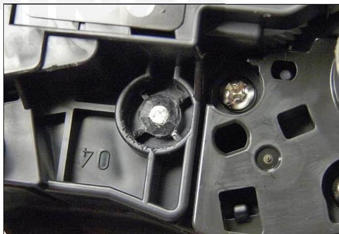
2. With a razor knife, carefully shave the plastic from the heads of the hinge pins on both sides of the cartridge.
