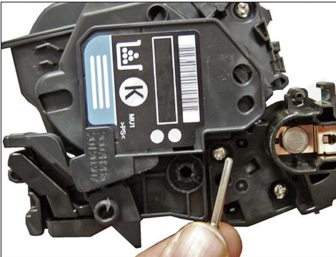
48. Install the two pins, large pin to the label or gear side of the cartridge.
