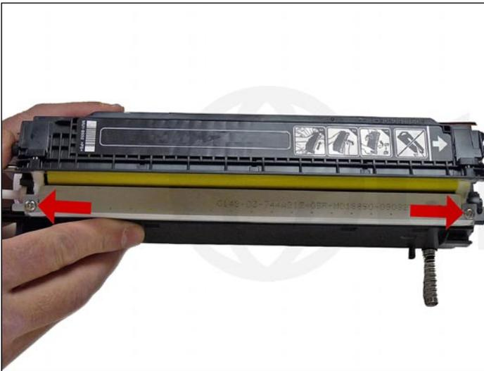
39. Use the appropriate shims to gap the blade and install the doctor blade and two screws. Make sure the adhesive seals on either end of the blade seal correctly. If the material is no longer sticky, clean it with alcohol or replace it with a small amount of silicon.
