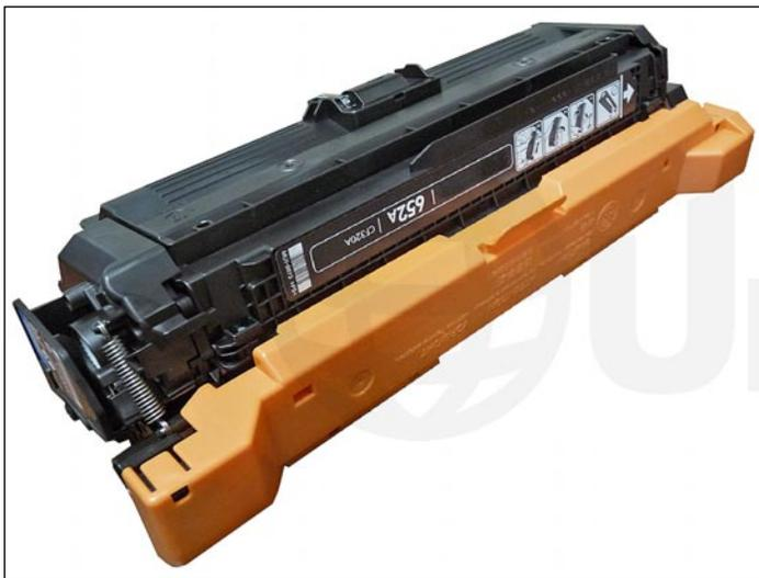
53. Install the drum cover on to the cartridge.
