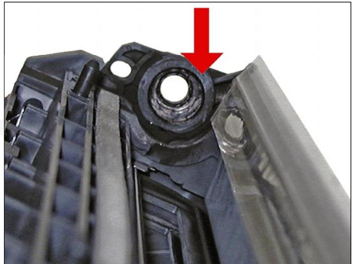
29. There are magnetic roller bushings on each side of the roller.
