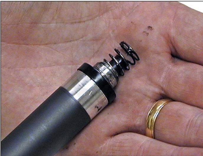
28. Note also the new heavy-duty style magnetic roller contact. This, when combined with the new larger diameter of the roller, allows the cartridge to run at the higher speeds that these machines are capable of.
