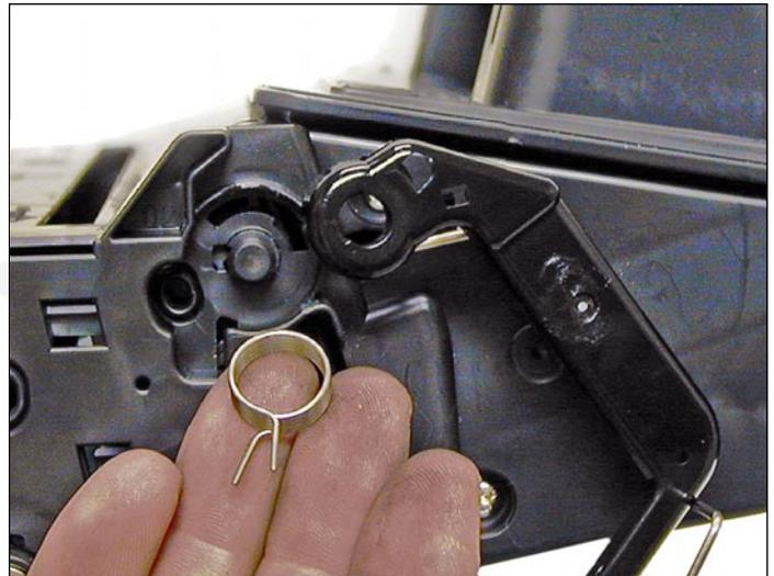
3. On the opposite side of the cartridge, carefully pry off the drum cover plastic arm. The spring will probably pop off, so take care not to lose it. We will go over the installation at the end of this article. Remove the drum cover assembly.
