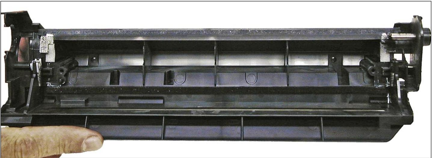
14. Due to the high speed and page counts of these cartridges, we recommend that the wiper blades be replaced.
