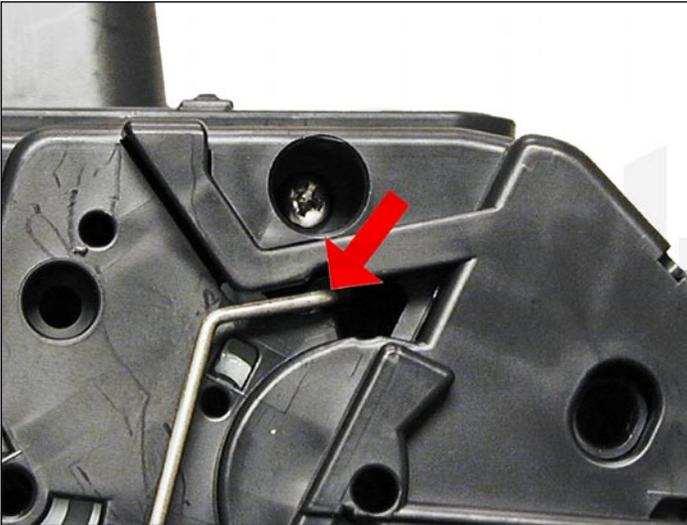
43. Install the metal bars from the drum cover on both sides of the cartridge.
