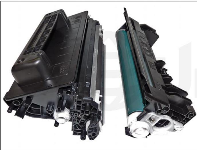
8. Separate the toner hopper and waste chamber.
