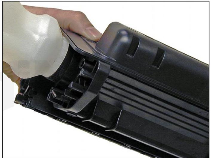
38. Fill with appropriate amount of toner for use in the M630 series. Install the fill plug.
