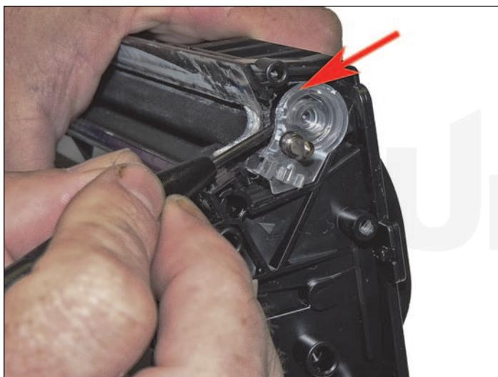
24. Carefully pry around the clear bushing that holds the feed roller in place. The plastic bushing can be removed by carefully prying it up with a small screwdriver from all around the edges. If you choose not to do this, you can melt a small hole in the supply chamber to clean the chamber out.
