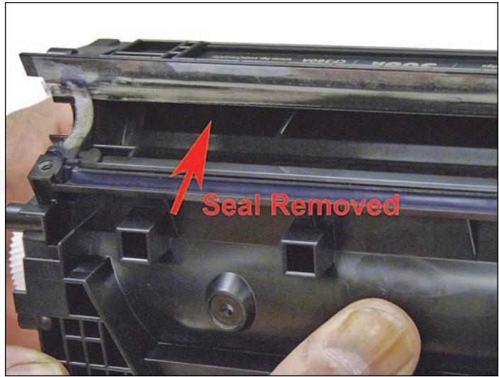
26. These cartridges have a self-removing seal that is not accessible from the outside of the hopper. Shown is a new hopper with and without the seal. To install a seal, it appears the hopper will have to be split. Testing is ongoing for this possibility.
