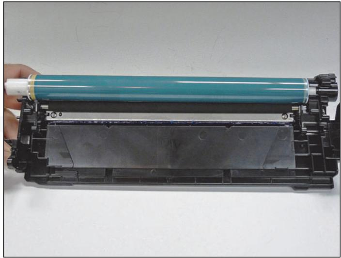
13. Clean and replace the conductive grease on the drum axle.
