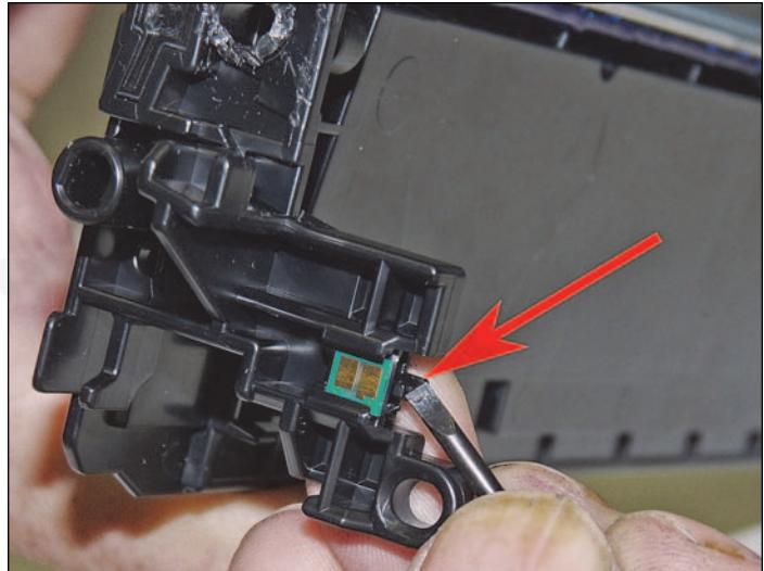
39. On the waste chamber, remove the chip by cutting the plastic off the edges of both sides of the chip and prying the locking tab back slightly.
