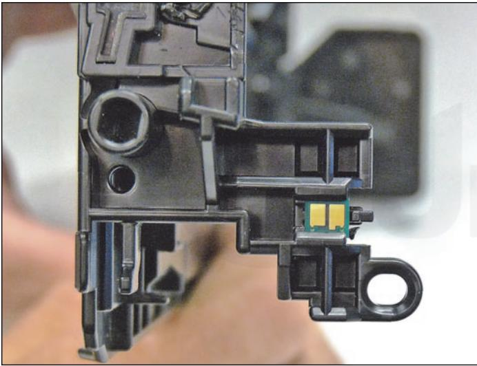
40. Remove and replace the chip. Make sure you have the correct color chip and the correct series!
