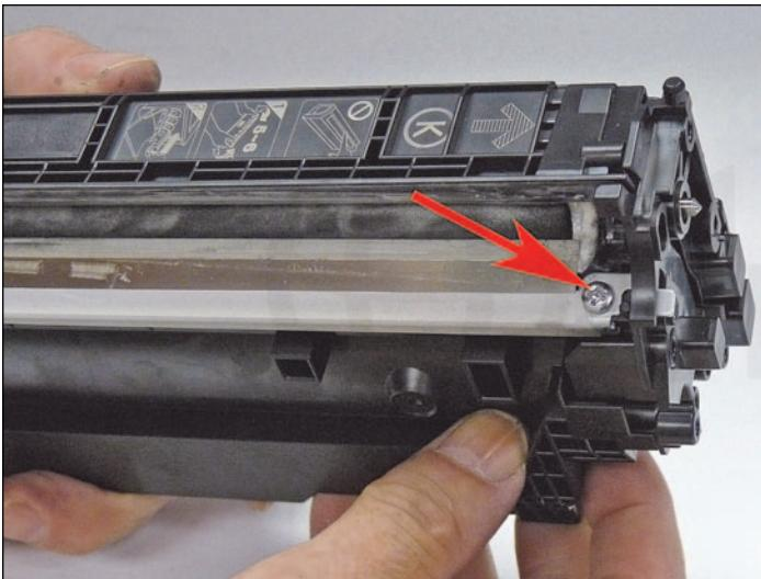
33. Install the left-hand doctor blade screw fully. This screw fits into a post on the inner end cap. The doctor blade is hard to install correctly if the inner end cap is already in place.
