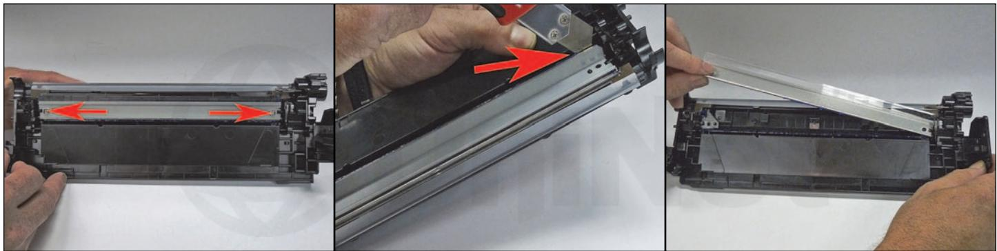
8. Remove the two screws from the wiper blade.
