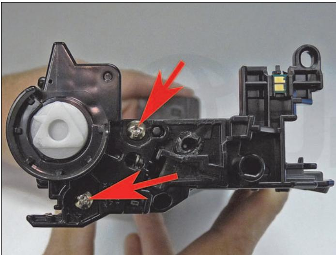
14. Install the end cap and two screws.
