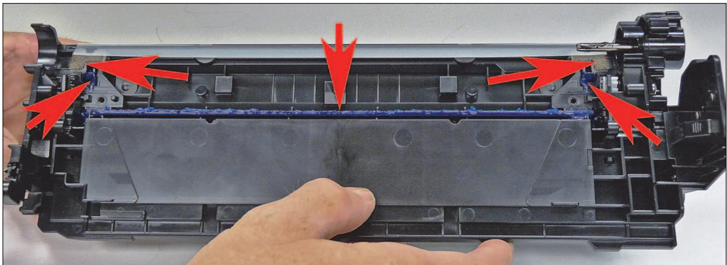
9. Clean out all the waste toner from the chamber. Try not to get any toner on the wiper blade seal if possible.
