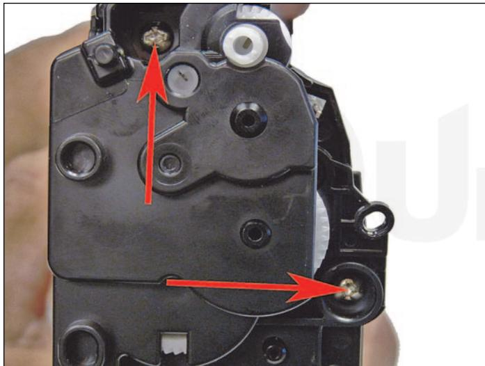
37. Install the gear end cap and two screws. You might have to turn the gears slightly for the end cap to fit in place.
