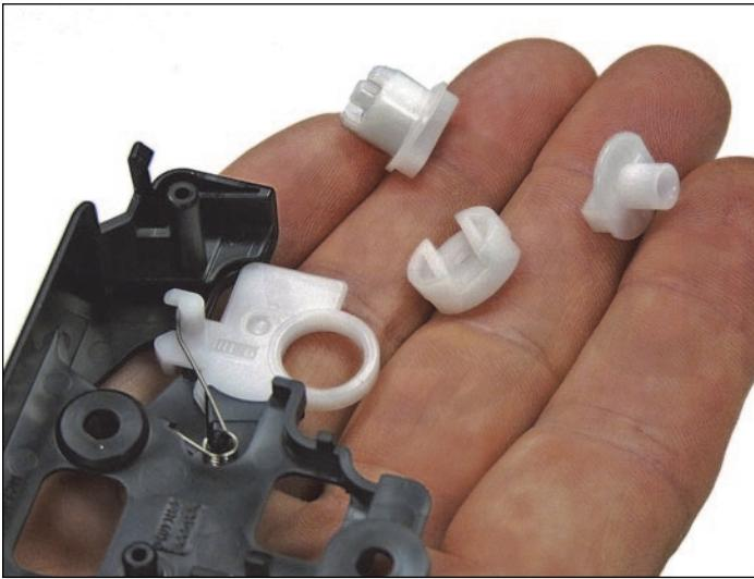
19. Remove the three developer roller drive gears.
