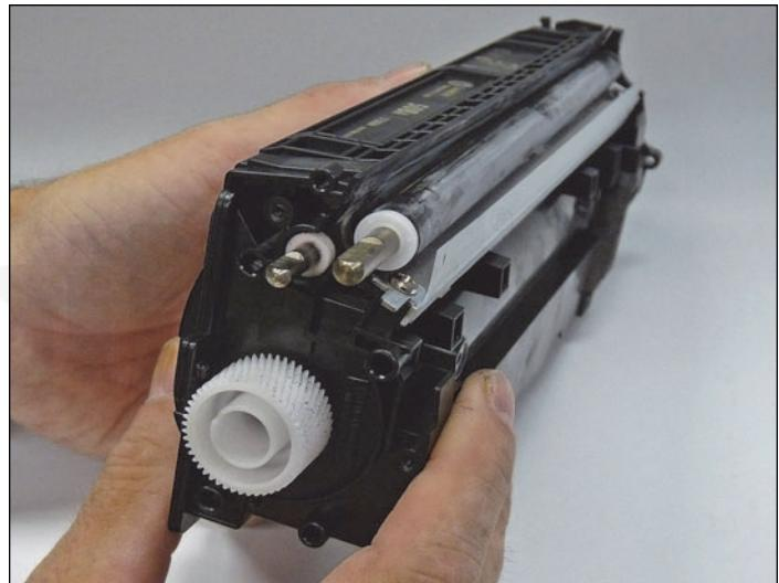
34. Install the cleaned developer roller, keyed-end to the gear side. Do NOT use any chemicals to clean this. A lint free cloth works fine.
