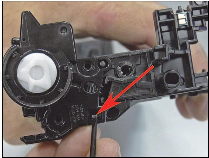
5. On the waste chamber, remove the two screws from the drum gear end cap.
