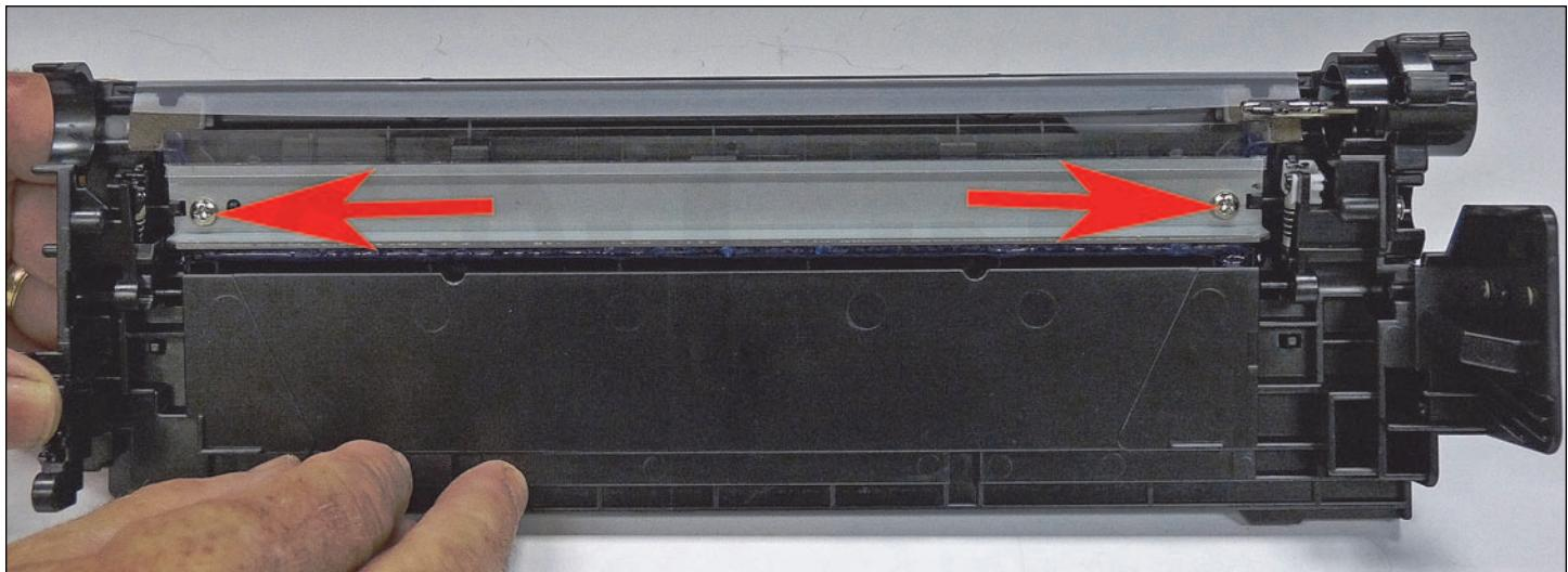
11. Install a new, lubricated wiper blade and two screws.
