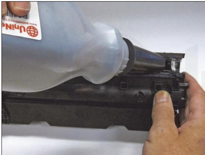
27. Clean out the remaining toner and fill with the correct color of toner for use in the M553 series toner.
