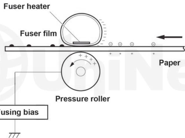
In the **fifth** stage, the image is then fused onto the paper by the fuser assembly. The fuser assembly is comprised of the upper heating assembly and lower pressure roller. The lower pressure roller presses the page up into the upper heating assembly, which then melts the toner into the paper. This heating assembly consists of a flexible sleeve with a ceramic heating coil inside. This type of fuser affords “instant on” fusing with little to no wait time, and low power consumption.
