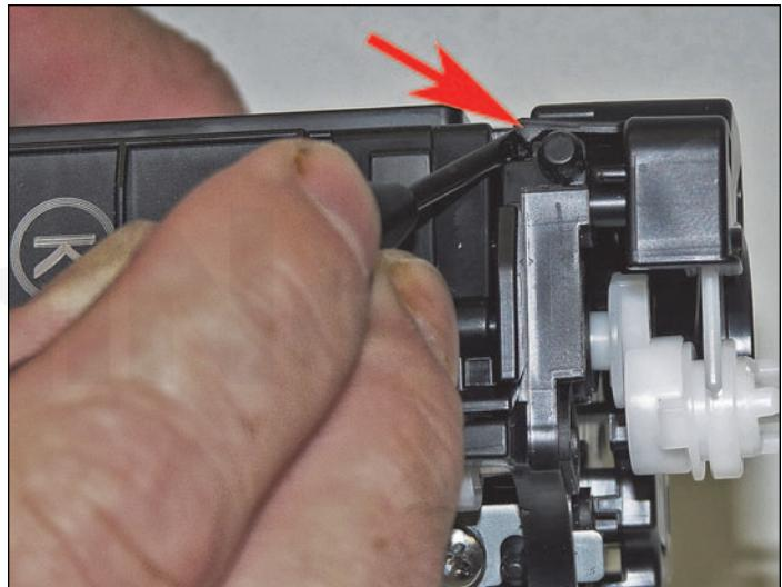
18. On the contact side, remove the two screws, pry out on the tab, and remove the end cap.
