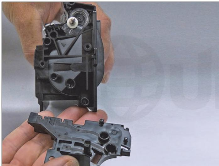
22. Remove the contact side inner end cap.
