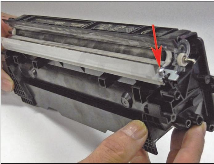
31. Use the appropriate shims to gap the blade and install the doctor blade and two screws. Make sure the sticky seals on either end of the blade seal correctly. If the material is no longer sticky, clean it with alcohol or replace it with a small amount of silicon. Leave the right side "left-hand screw" partially installed.
