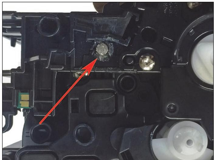
2. With a razor knife, carefully shave the plastic from the heads of the hinge pins on both sides of the cartridge.
