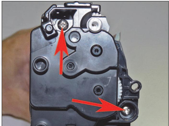
16. On the supply chamber, remove the two screws from the gear side end cap.
