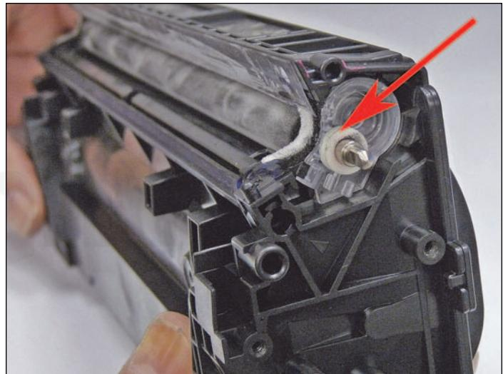
29. Install the clear plastic bushing. Use a very small amount of a silicon sealer to make sure there are no leaks. Be careful to keep the silicon around the outside edges.
