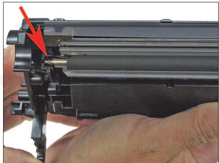
12. Clean the PCR with your preferred cleaner and install in the cartridge. Note there is conductive grease on both sides of the PCR axle. If worn or dirty, clean the axles and holder with alcohol and replace with conductive grease. Replace with the same amount that was there. More is NOT better!
