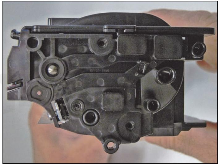
32. Install the inner contact end cap.
