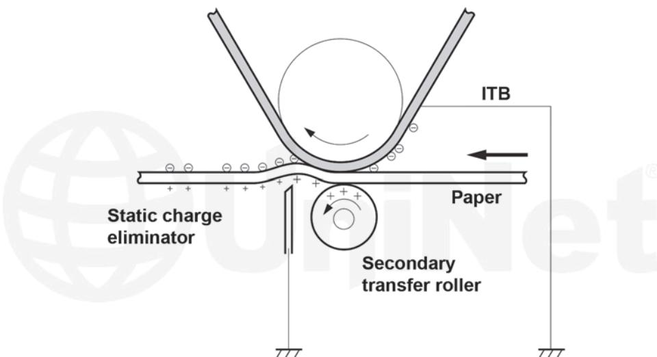
The paper separates from the ITB belt as the belt turns back down to start the process again. The static charge on the back of the paper is decreased with static charge eliminator. This helps stabilize the paper feed, and also prevents toner flares (spots) under low temperature and low humidity conditions.
