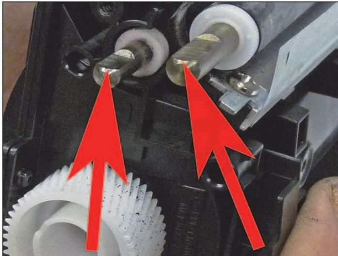
35. Set the developer roller shaft and feed roller shafts as shown (flat side up).
