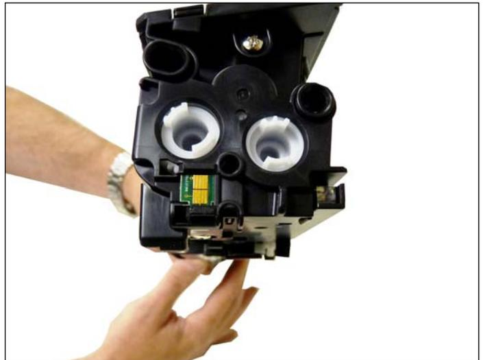
15. Slide the fill side end cap in place. Install the screw and replace the label (the label as you can see is easily torn).
