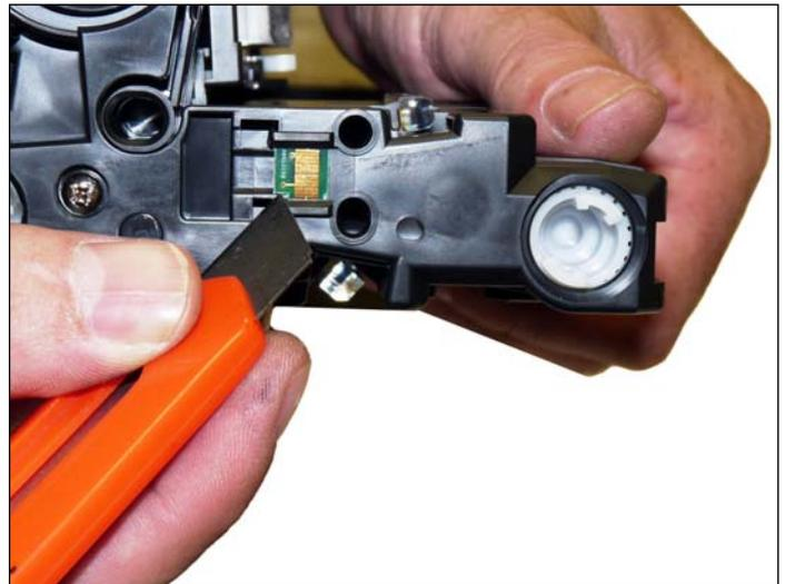
40. Replace the chip by slicing the melted plastic from the top edge. Slide the chip out and replace. Lock the replacement chip in with two small dots of hot glue.
