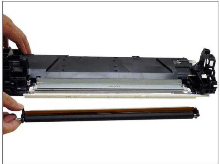
16. Remove the PCR assembly. The film will come with it.
