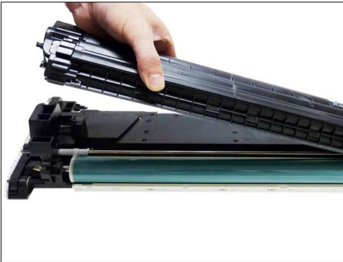
6. Lift the developer unit off the cartridge.
