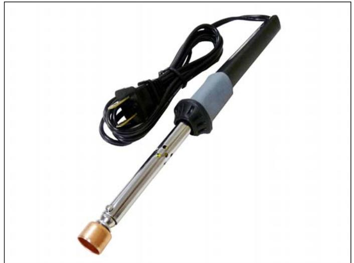
1. The toner cartridge does not have a fill plug or an opening large enough to clean or refill it through. Because of this, the cartridge needs to have a hole cut. This is best done with a soldering iron with a screw in tip and a 1/2" copper plumbing end cap drilled, filed and screwed on the iron. You can also drill the hole, but you must be very careful not to get plastic shavings inside the cartridge.
