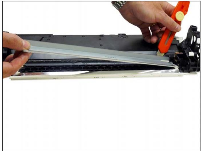
18. Remove the two screws on the wiper blade. Carefully pry up the blade carefully cutting the wiper blade seal as you go.
