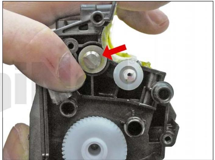
29. Remove the felt washers from both sides of the feed roller.
