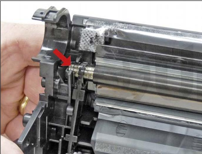
15. Place conductive grease on the black holder side of the shaft.
