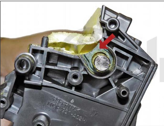
35. Install the feed roller and rubber bushing, with the keyed end to the gear side.
