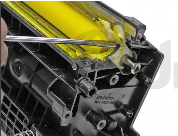
28. On the right side of the chamber, lift up the felt developer roller seal. Lift it from the front side and lay it over the back.
