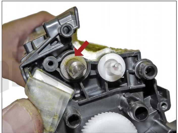
36. Install the feed roller felt washers.
