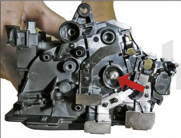
39. Clean the contacts and replace the conductive grease on the inner contact end cap. Install the inner contact end cap and screw.
