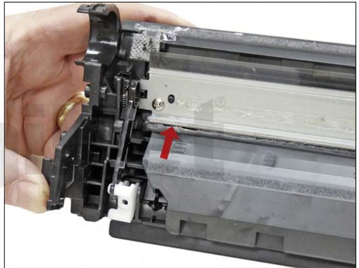
12. Install the new wiper blade and two screws.
