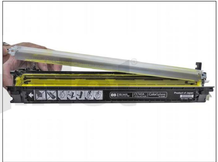
27. Remove the two screws from the doctor blade and start to lift the blade up.
