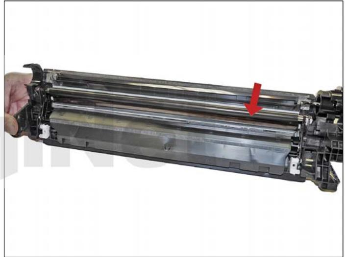
14. Clean the PCR with your preferred cleaner and install in the cartridge with the PCR holders. Make sure you lock the locking arms in place.
