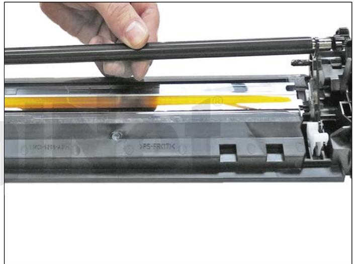
8. Remove the PCR by lifting up on the black and white PCR locking arms. Remove the PCR, the arms will stay in place.
