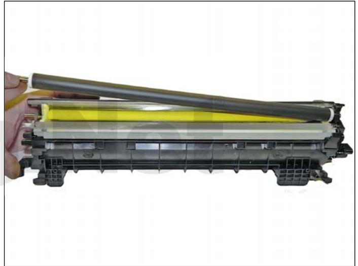
40. Install the cleaned developer roller. Do not use any chemicals to clean this. A lint-free cloth works fine. Place the keyed end to the gear side and conductive grease on the contact side.
