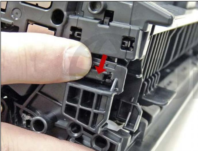
4. On the gear side, press in on the plastic locking mechanism.
