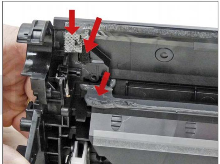
11. Clean the felt seals on each end of the wiper blade. If the wiper blade glue has toner on it, clean it off with alcohol and a foam swab. If it does not become sticky again, it needs to be removed and a good silicone caulk used to seal the blade off. GE 100% silicone and Phenoseal are two good brands for this.
