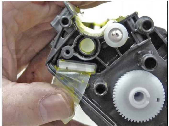
34. Remove the seal port and slide the seal pull tab through the slot.
