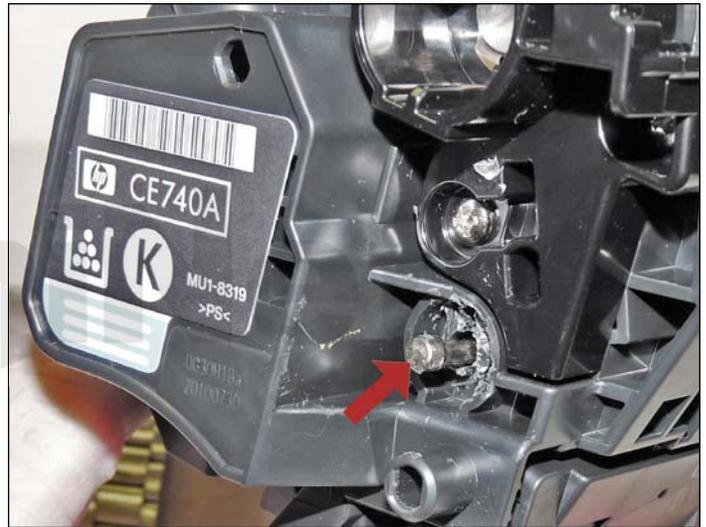
3. Remove the pins with flush cutting wire cutters.
