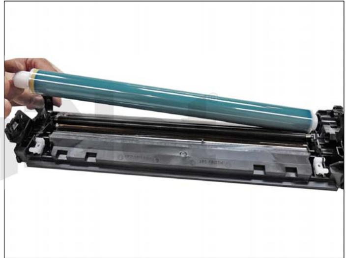
16. Install the drum (short hub side) onto the long drum ground/axle pin. Make sure there is conductive grease on the drum ground/axle pin.
