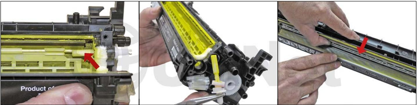
33. When a seal is available, you will first need to remove the auger drive gear and remove the auger so that you have access to the seal area. Install the seal onto the seal rails. Pull the release tape off 1" at a time and press the seal in place as you go. Install the auger and auger drive gear. Make sure the drive gear is positioned as shown.
