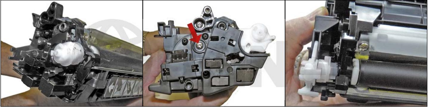
44. Place the triple gear on the developer roller shaft, and fit into the spring assembly on the end cap.
