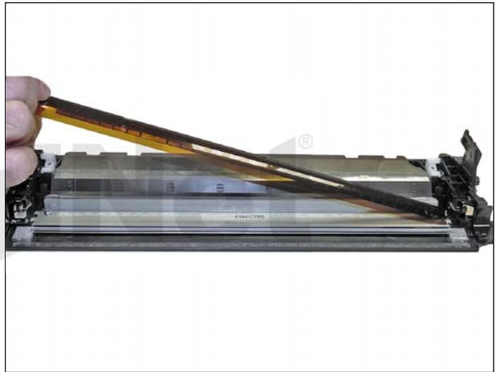
9. To remove the wiper blade, the amber film assembly needs to be removed.
