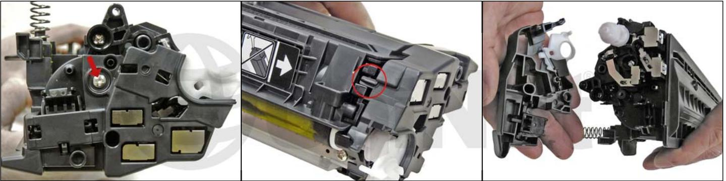
22. On the contact side, remove the screw, pry up on the small tab and remove the end cap.
