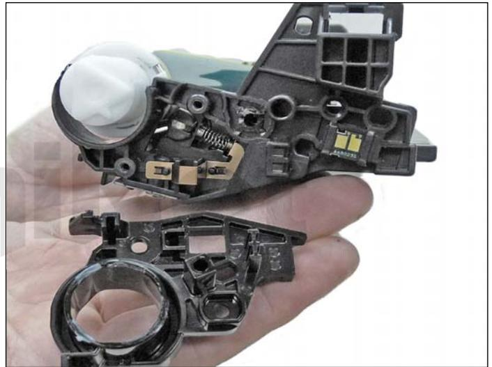
6. On the waste chamber, remove the two screws from the drum gear end cap.
