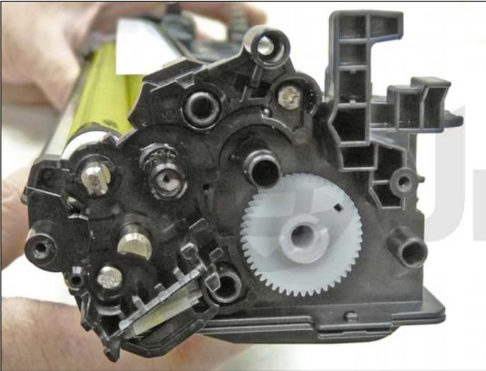
21. Remove all the gears as shown except for the mixing blade gear and the sealing strip gear. The mixing blade gear is attached to the mixing blade inside the hopper and is very difficult to re-attach properly.
