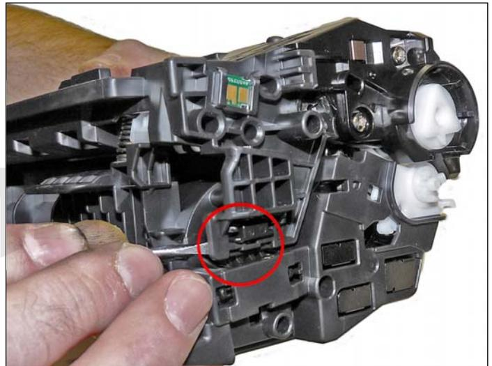
45. Place the two halves together with contact side first.
