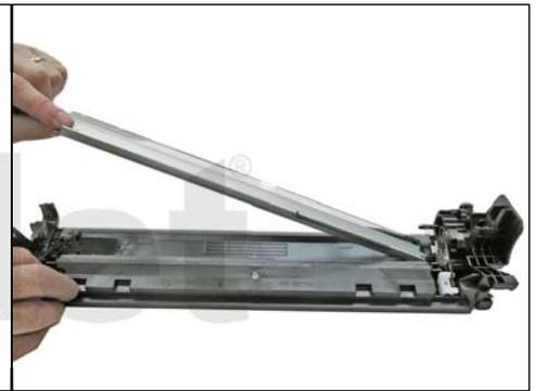
10. Remove the two screws from the wiper blade. Slide the razor knife along the back edge of the blade to release it from the glue. Remove the wiper blade. Clean out all the waste toner from the chamber. Try not to get any toner on the wiper blade seal if possible.
