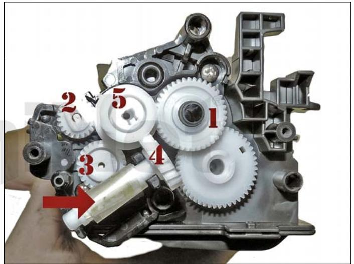
42. Install the gears in the order shown. If you installed a seal, slide the seal end through the take up gear and wrap the loose tail tight on the roller.
