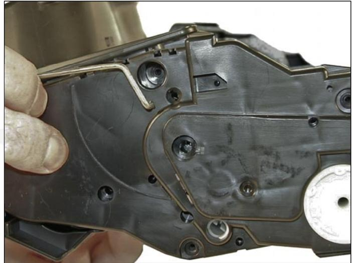
3. Open the drum cover towards the back of the cartridge.
