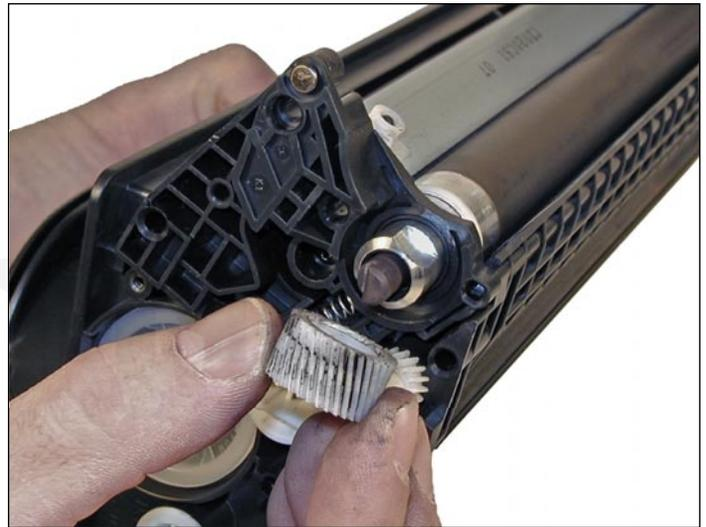
37. Install the magnetic roller sleeve drive gear.
