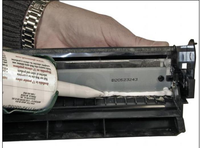
17. Seal the back edge of the wiper blade with a good quality silicon caulk. Use the type that never dries (cannot be painted).
