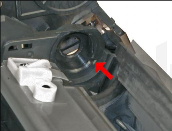
33. On the magnetic roller sleeve, there is a small hub that is keyed into its holder. Align and install the hub with its slot, as well as the entire magnetic roller sleeve assembly.
