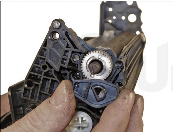
38. Install the keyed magnetic roller sleeve cover. Make sure that the keyed hole in the cover matches the keyed end of the magnet in the magnetic roller sleeve assembly.
