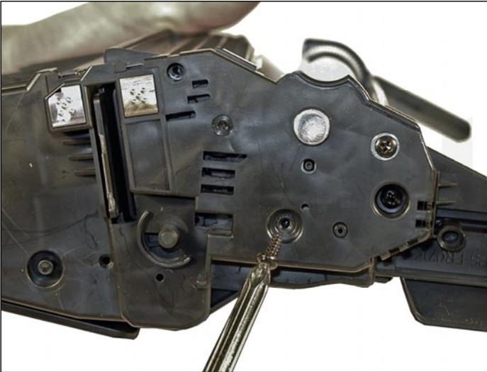
40. Install the two screws into the end cap.
