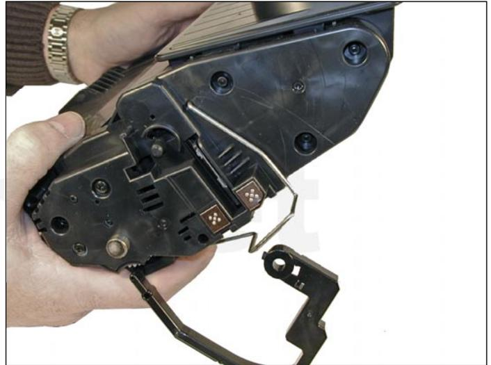
43. Install the metal bars from the drum cover on both sides of the cartridge. You will have to turn the bars so that the flattened end of the bars fit into the keyed slots.
