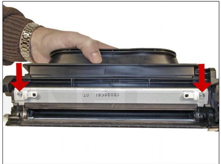
32. Install the doctor blade and two screws. Make sure that all the spacers (both clear and white) are seated correctly!
