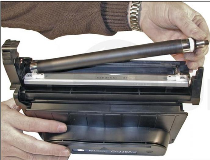
24. Remove the magnetic roller sleeve assembly.
