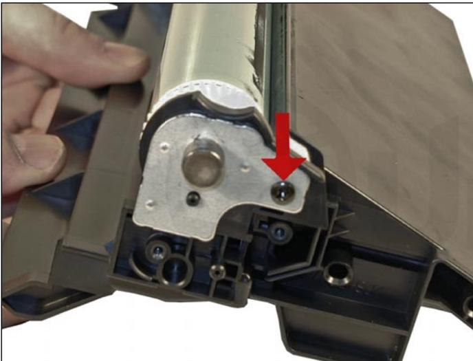
9. Remove the metal drum axle pin screw and the axle pin.
