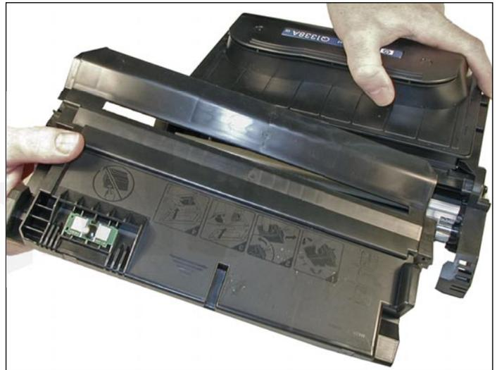
8. Carefully work the waste chamber loose from the right side end cap. Press in on the metal drum axle pin to help free it.
