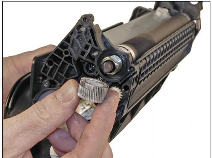
22. Remove the magnetic roller sleeve drive gear.
