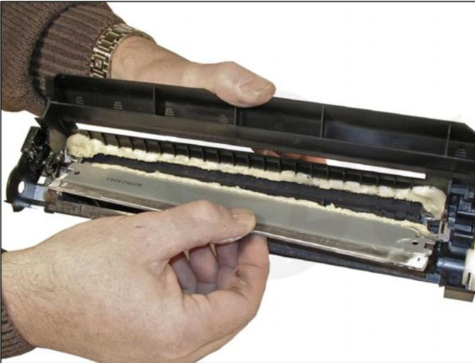
13. With a razor knife, carefully lift up the seal foam and cut away. This is very sticky stuff, the best way to remove it is to cut and lift.
