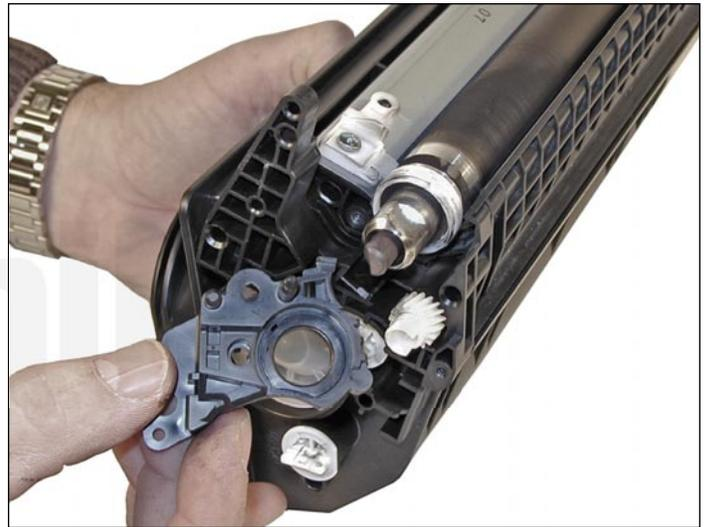
23. Note the location of the spring that sits between the magnetic roller sleeve holder and the hopper.
