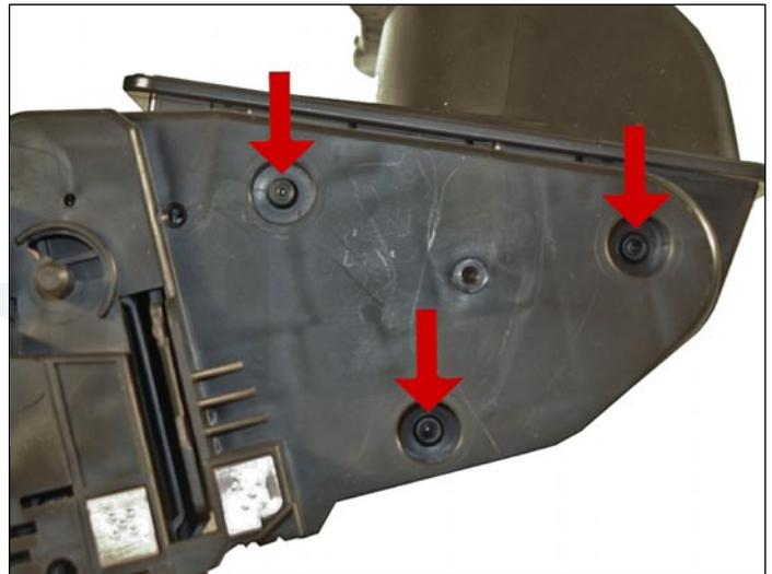
The rest of the right side end cap is held in place by three melted plastic posts.
