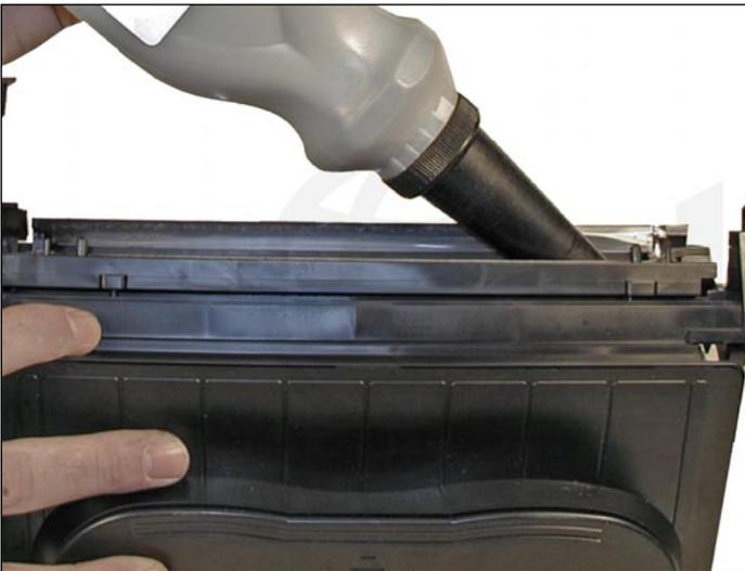
31. Fill with 690g of replacement polyester-based toner for use in HP 4200, or 1,100g for use in HP 4300 cartridge.
