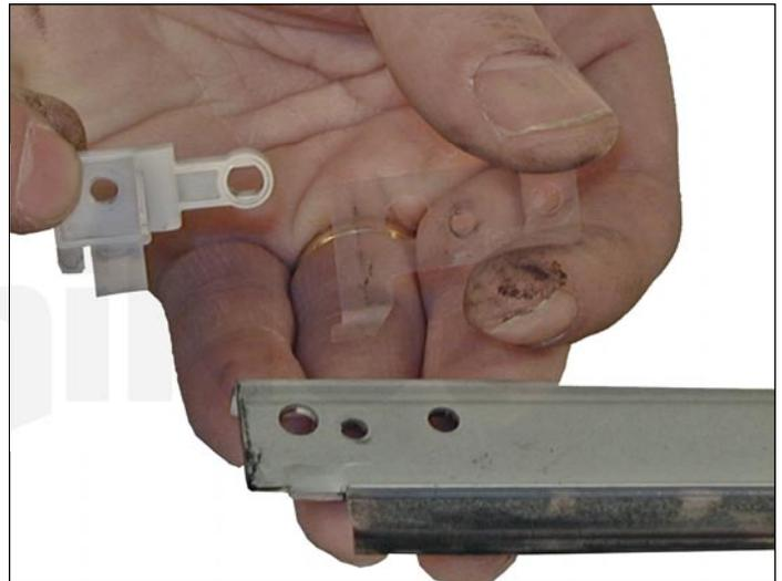
25. Remove the two doctor blade screws and the doctor blade.
