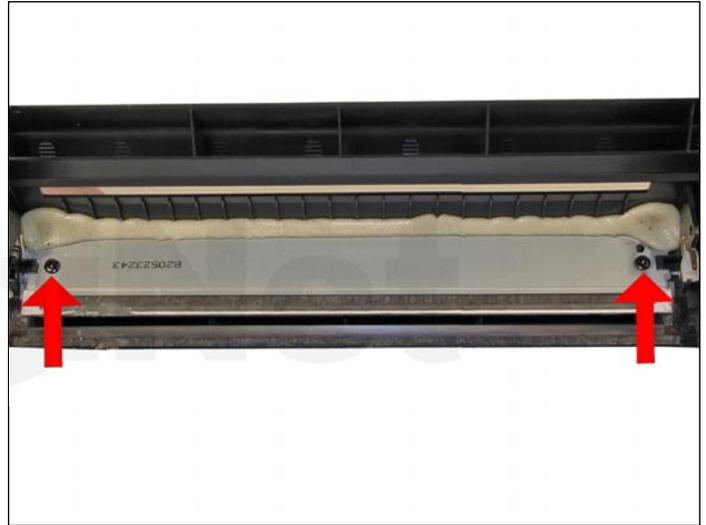
12. Remove the two screws from the wiper blade.
