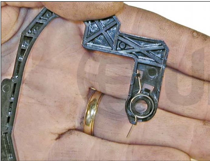
40. Install the spring into the drum cover arm as shown. Pull the upper tail of the spring until it fits into the notch in the arm hub.
