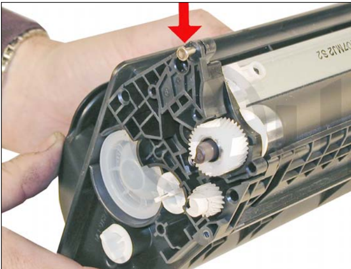
20. Remove the small metal pin from the MRS holder.
