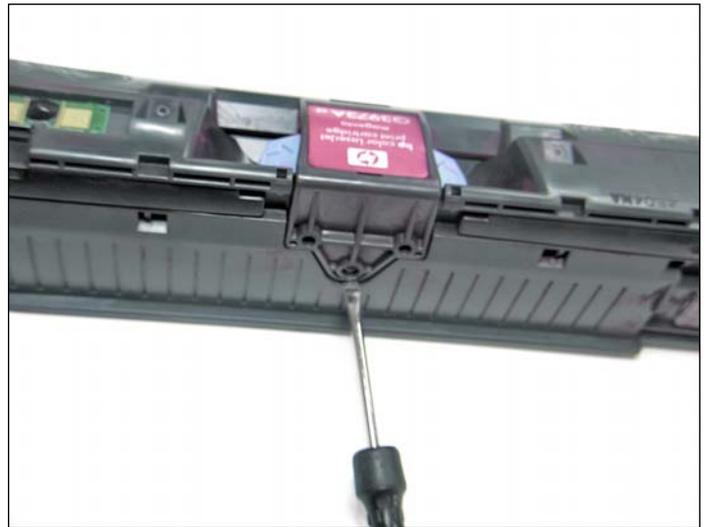
12 Use a small flathead screwdriver to pry off the back of the doctor blade cover as shown.
