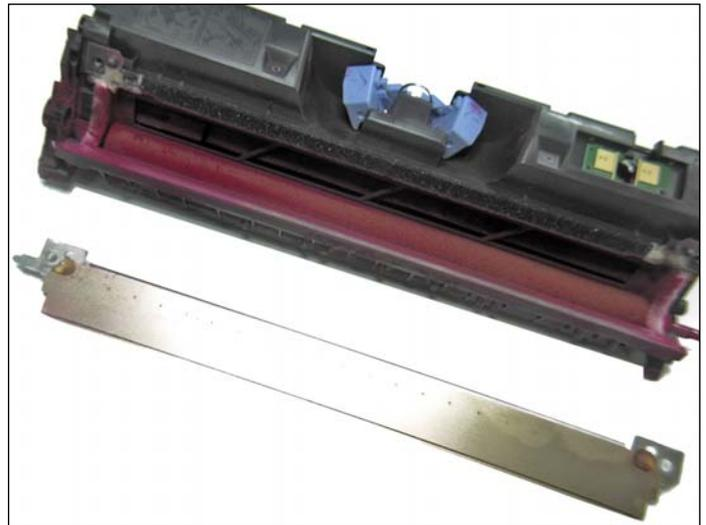
16. Remove the doctor blade. Be careful not to lose the small spring at the end of the doctor blade.
