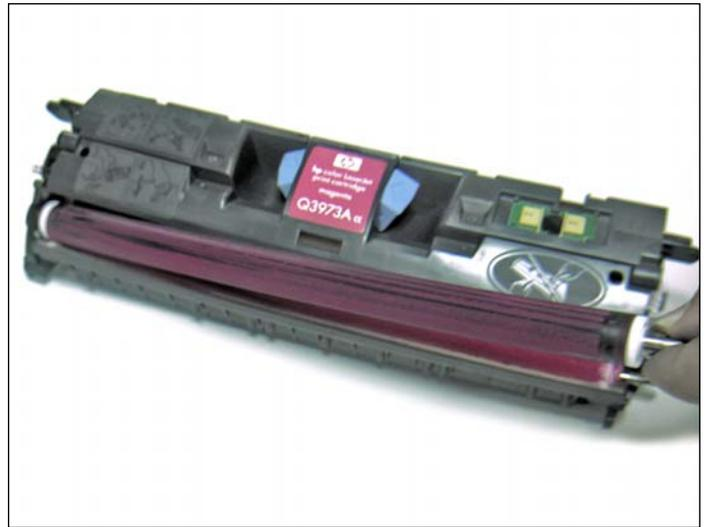
10. Remove the developer roller as shown.
