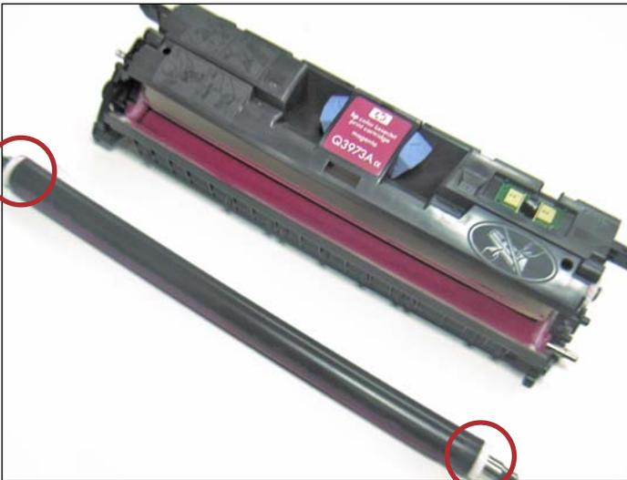
11. Be careful not to lose the white bearings located at the ends of the developer roller.
