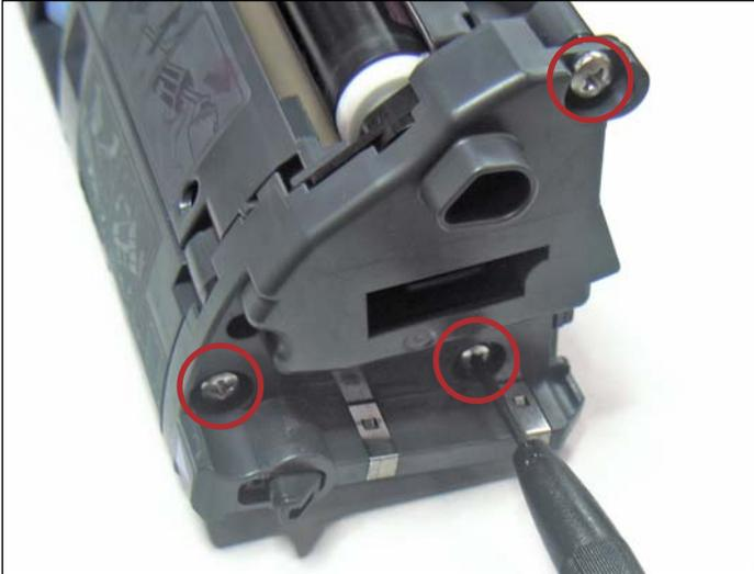
1. Remove the three screws on the non-gear side end cap.
