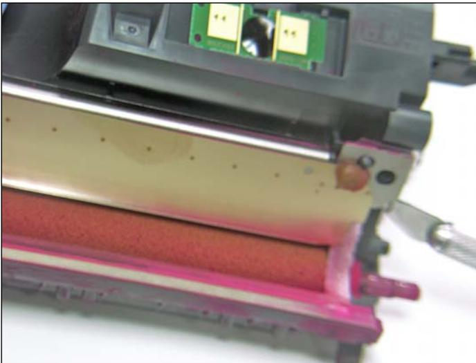
15. Using an X-acto knife, carefully cut away the adhesive gum on the back ends of the doctor blade to loosen them.
