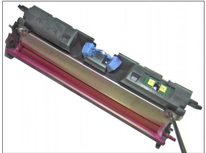
14. Remove the two screws on the ends of the doctor blade.
