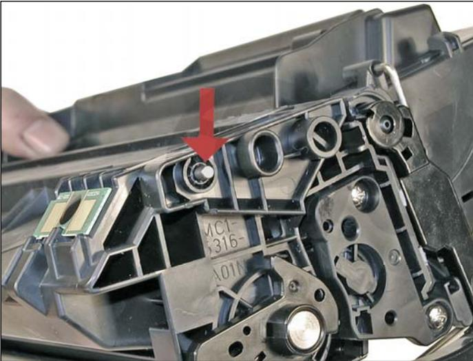
21. Place the two halves together and insert the two silver pins.
