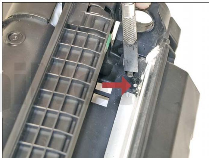
5. Take the X-Acto knife with the chisel blade and cut the pin cover off by slicing it at the side wall of the cartridge.
