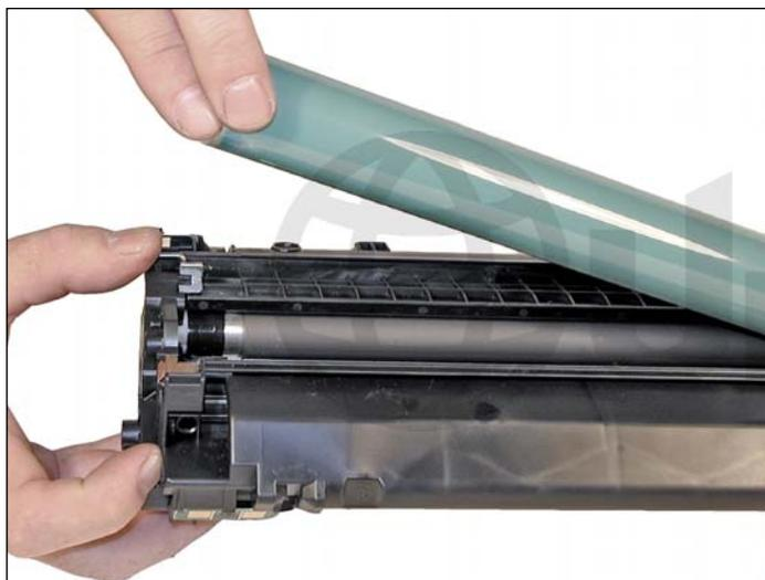
3. Hold the two halves slightly apart and remove the photoconductive drum being extremely careful not to scratch it. If the drum is in good shape and you plan to reuse it, blow off any toner and debris from drum, being careful not to let the air gun come in contact with the drum surface. Do not polish or wipe the drum with a dry cloth, since this may scratch the drum.
