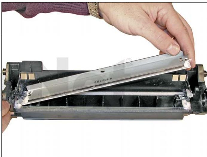
8. Due to the aggressive nature of the toner used in these cartridges, we recommend that the wiper blade be replaced each cycle. Lightly coat the new blade with Kynar drum padding powder. Replace the wiper blade into the cartridge.
