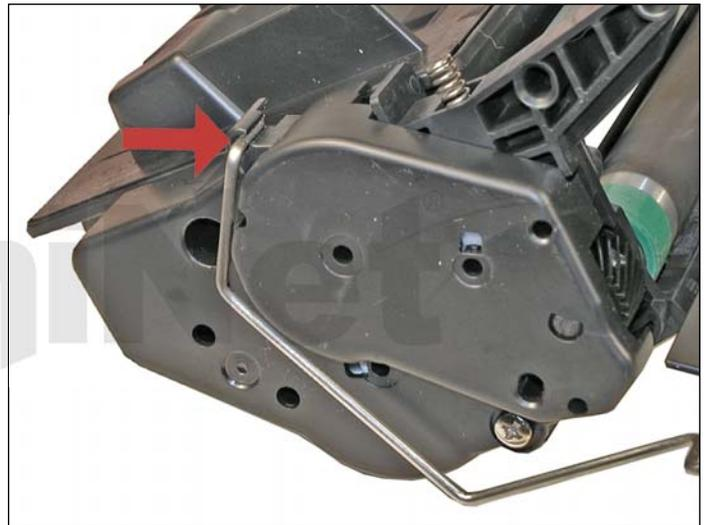
20. Install the metal bars on both sides.
