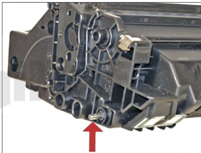
6. This will give you access to the pins where you can take the small punch or a small screwdriver, and gently press both of the metal pins out from the inside of the cartridge. To make this process easier, push the pins out halfway, and pull them out from the outside with needle nose pliers or wire cutters. The pins will move out enough to grab them with pliers from the outside.
