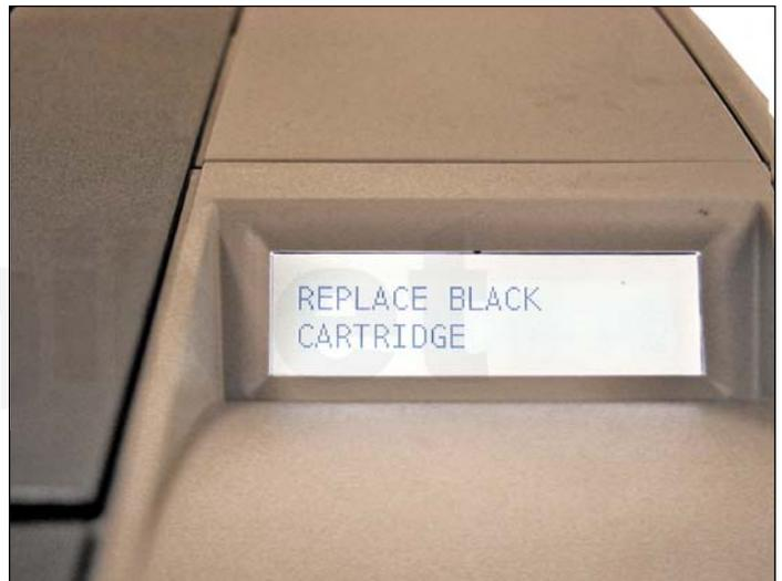
Shown here is the display panel when a cartridge is inserted with a used chip.
