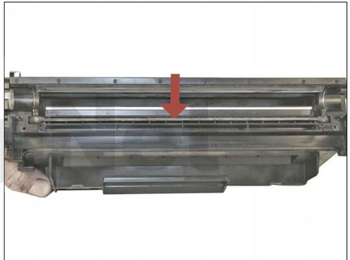
11. Remove the doctor blade by removing the two screws and lifting it out straight up. When removing this blade, be very careful not to break the alignment pins. These pins keep the doctor blade at the proper distance from the magnetic roller. There is a thin bead on adhesive under the blade. Be sure to keep it clean so that it stays sticky.
