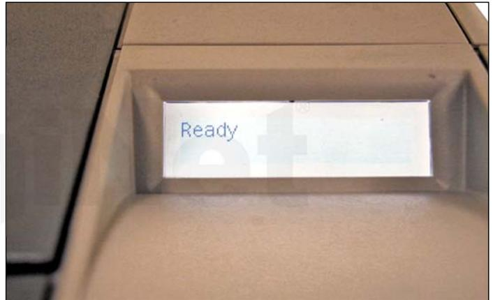
As with all other black HP cartridges, the chips on these cartridges do not shut down the entire cartridge, they disable the “toner low” features. The cartridge will run if the chip is removed, but the error message must be cleared first. As with past HP chips, the toner low function is disabled if a used chip is installed. Shown above is the display panel when a cartridge is inserted in the printer with a no chip.
