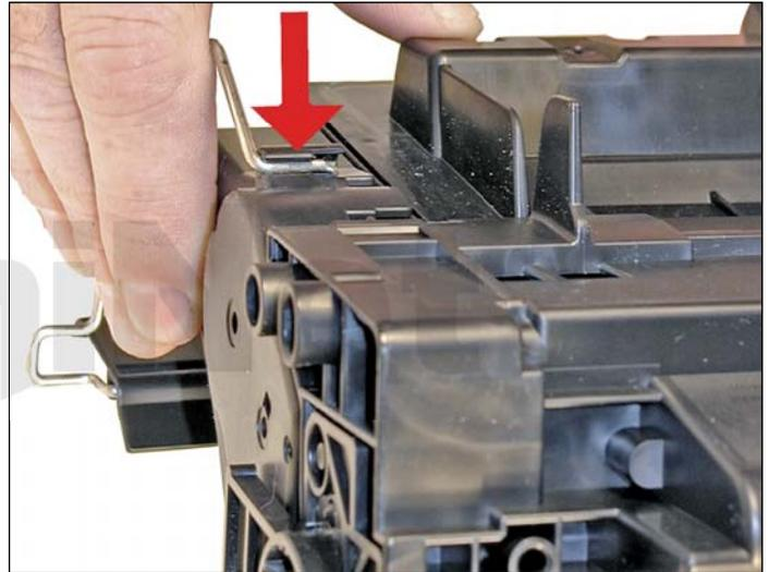
1. Remove the drum cover by prying the spring-loaded arm, and then carefully pry off the two metal bars out of their holders.
