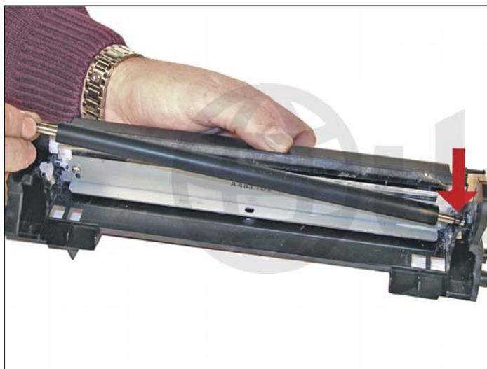
9. Place a small amount of conductive grease on the black PCR holder, and install the PCR. Place the waste chamber aside.
