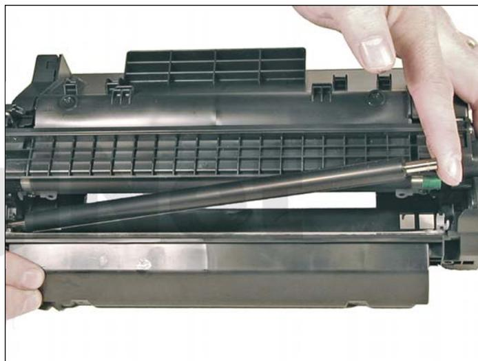
4. Carefully remove the primary charge roller (PCR), by gently prying it out of the clips on either end. Be careful as the PCR holders come loose easily! Place the PCR aside.
