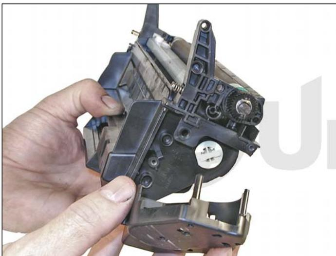
17. Install the large end cap and two screws.
