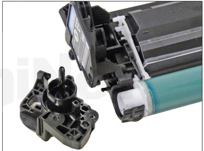
8. Remove the two screws from the contact side end cap.
