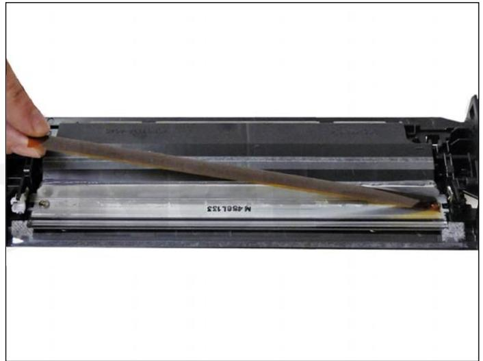
11. To remove the wiper blade, the amber film assembly needs to be removed.
