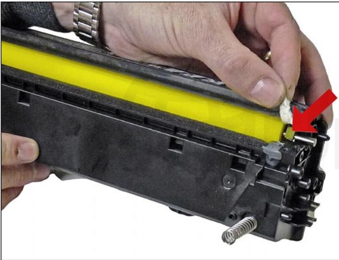
36. Install the feed roller and bushing.
