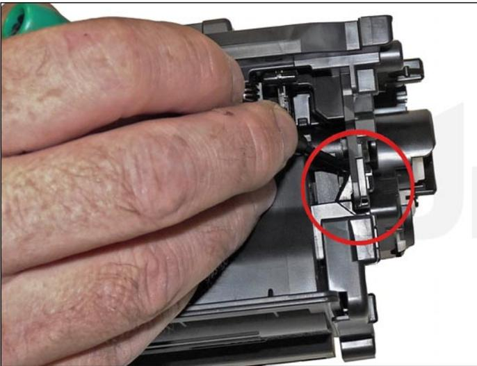
47. Place the two halves together, contact side first.
