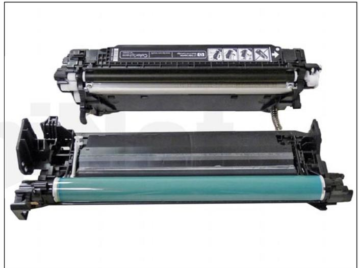
6. On the opposite side lift up on the waste chamber until the two halves separate.
