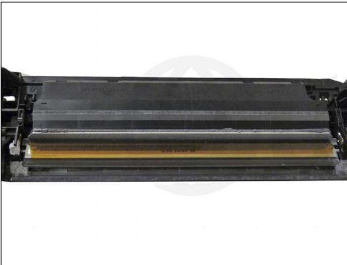
16. The amber film assembly is held in place with double-sided tape. If this is not sticking, remove the old with alcohol and replace. Replace the film assembly.
