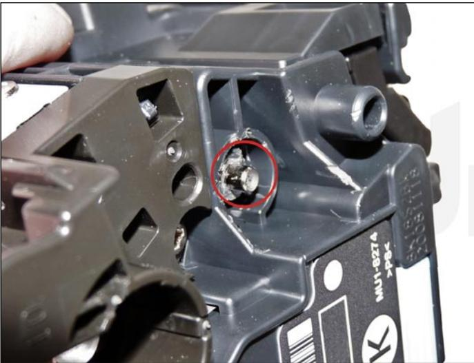
4. Push the pins out with a jeweler's screwdriver. With the hole in this location, and by just pushing the screwdriver in, the pins will be pushed out. Remove the pins. The gear side has the smaller of the two pins.
